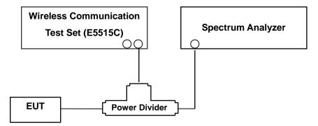
(Configuration of conducted Emission measurement) Test Procedure
