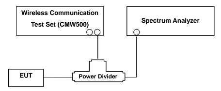
(Configuration of conducted Emission measurement) Test Procedure
