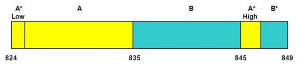
BLOCK 1: 824 – 835 MHz (A\* Low + A) BLOCK 2: 835 – 845 MHz (B) BLOCK 3: 845 – 846.5 MHz (A\* High) BLOCK 4: 846.5 – 849 MHz (B\*)
