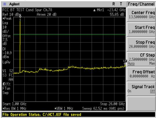
Test Plots (8DPSK) - 1 GHz - 26 GHz (RBW:1 MHz, VBW: 1 MHz) Spurious Emission (Low-CH)
