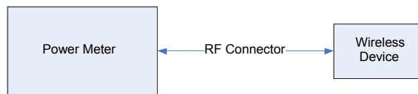
Figure 12-2 Power Measurement Setup
