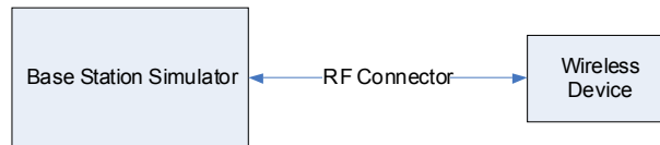
Figure 12-1 Power Measurement Setup
