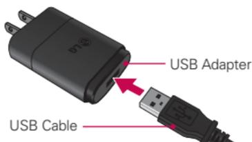
**NOTE** Make sure the battery is installed before connecting the USB adapter. If the battery is not installed and the USB adapter is connected, the phone will not operate properly due to prolonged power cycling. Also, removing the battery with the USB adapter connected may damage the device. Please unplug USB adapter before removing battery.
