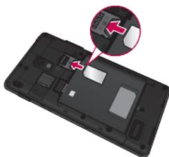
3. Insert the battery into place by aligning the gold contacts on the phone and the battery ❶ and press the battery down until it clicks into place ❷.
