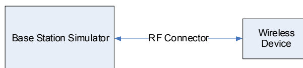
Figure 9-2 Power Measurement Setup
