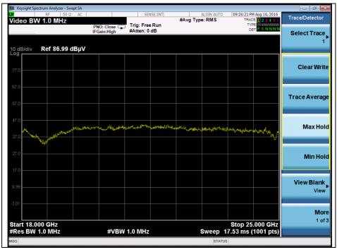
**Note:** Emission was scanned up to 25 GHz, No emissions were detected above the noise floor which was at least 20 dB below the specification limit.
