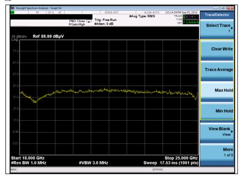
Note: Emission was scanned up to 25 GHz, No emissions were detected above the noise floor which was at least 20  ${
