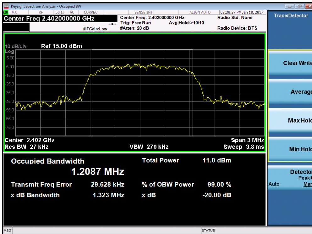
Plot 7-7. 20dB Bandwidth Plot (Bluetooth, 3Mbps – Ch. 0)
