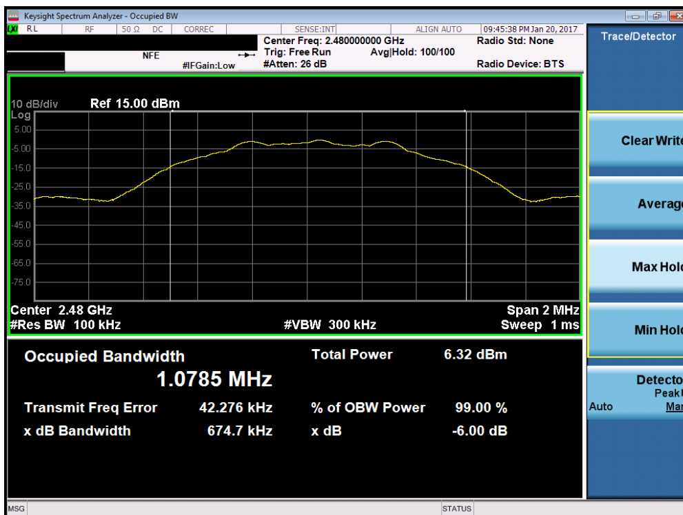
Plot 7-3. 6dB Bandwidth Plot (Bluetooth (LE) – Ch. 39)
