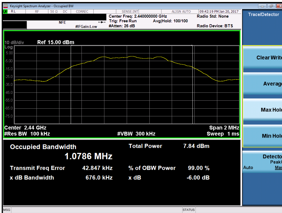
Plot 7-2. 6dB Bandwidth Plot (Bluetooth (LE) – Ch. 19)
