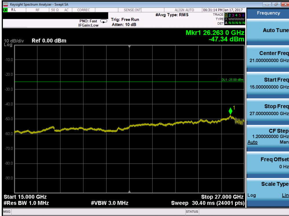
Plot 7-123. Conducted Spurious Plot (Band 7 – 10.0MHz QPSK – RB Size 1, RB Offset 0 – High Channel)
