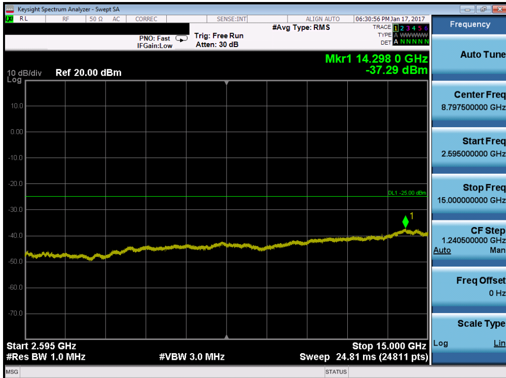
Plot 7-122. Conducted Spurious Plot (Band 7 – 10.0MHz QPSK – RB Size 1, RB Offset 0 – High Channel)
