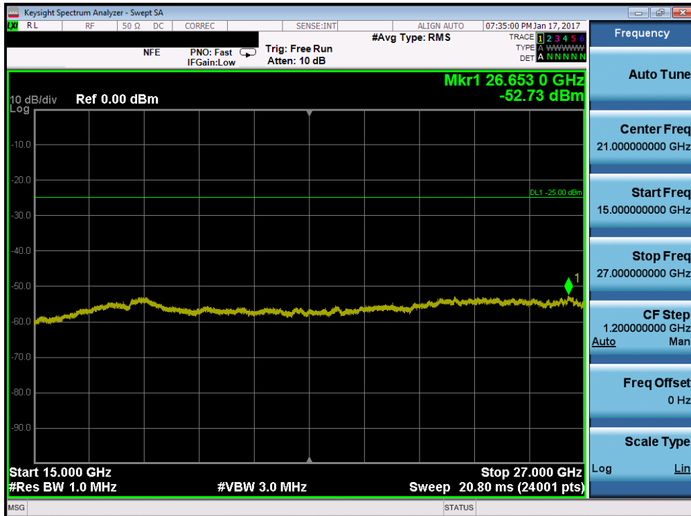
Plot 7-120. Conducted Spurious Plot (Band 7 – 10.0MHz QPSK – RB Size 1, RB Offset 0 – Mid Channel)
