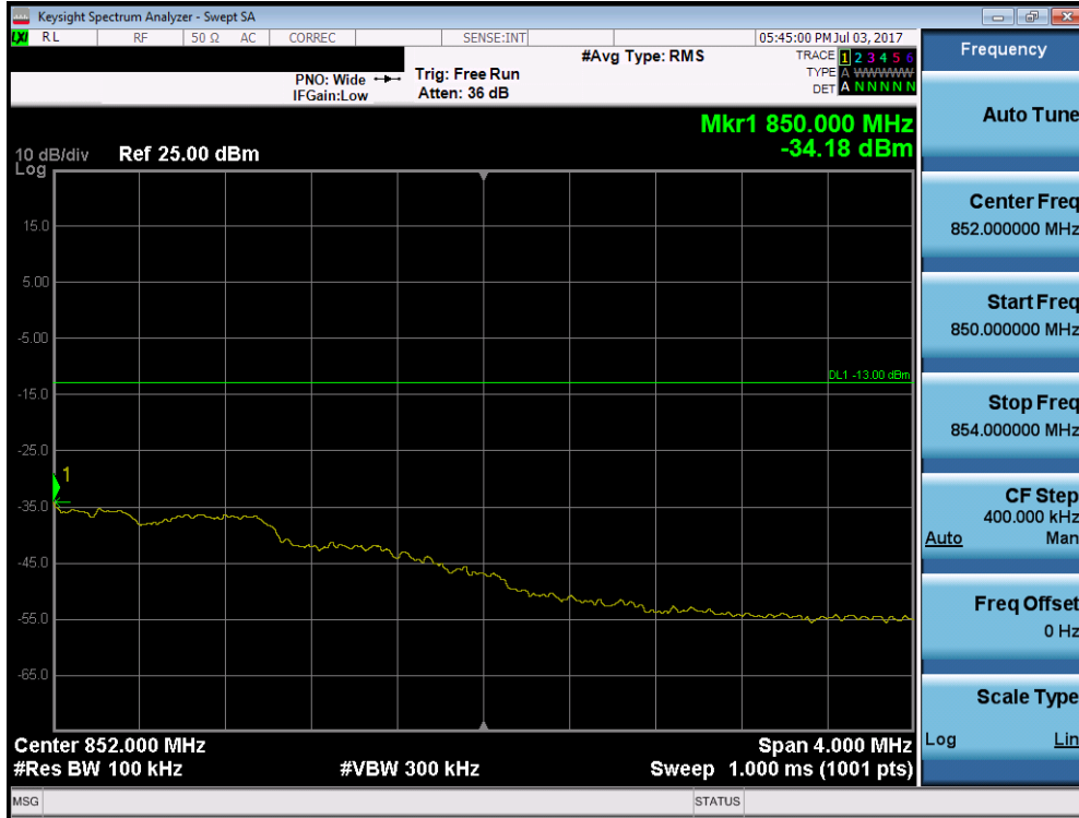
Plot 7-109. Upper Extended Band Edge Plot (Band 5 – 1.4MHz QPSK – RB Size 6)
