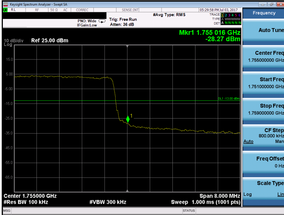
Plot 7-123. Upper Band Edge Plot (Band 4 – 10.0MHz QPSK – RB Size 50)
