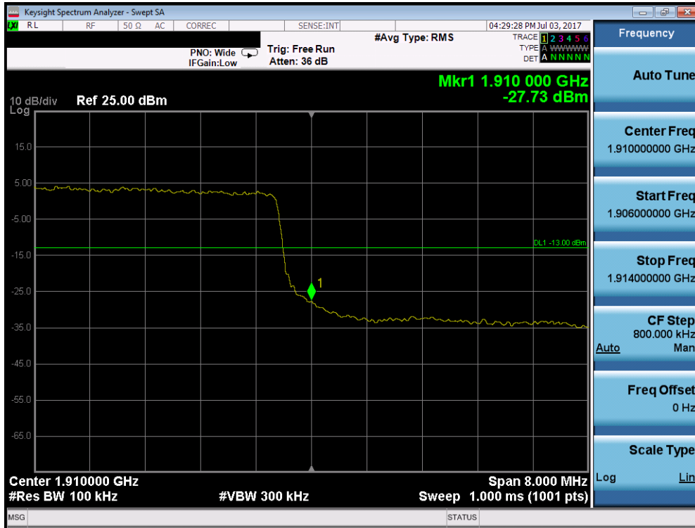
Plot 7-167. Upper Band Edge Plot (Band 2 – 10.0MHz QPSK – RB Size 50)
