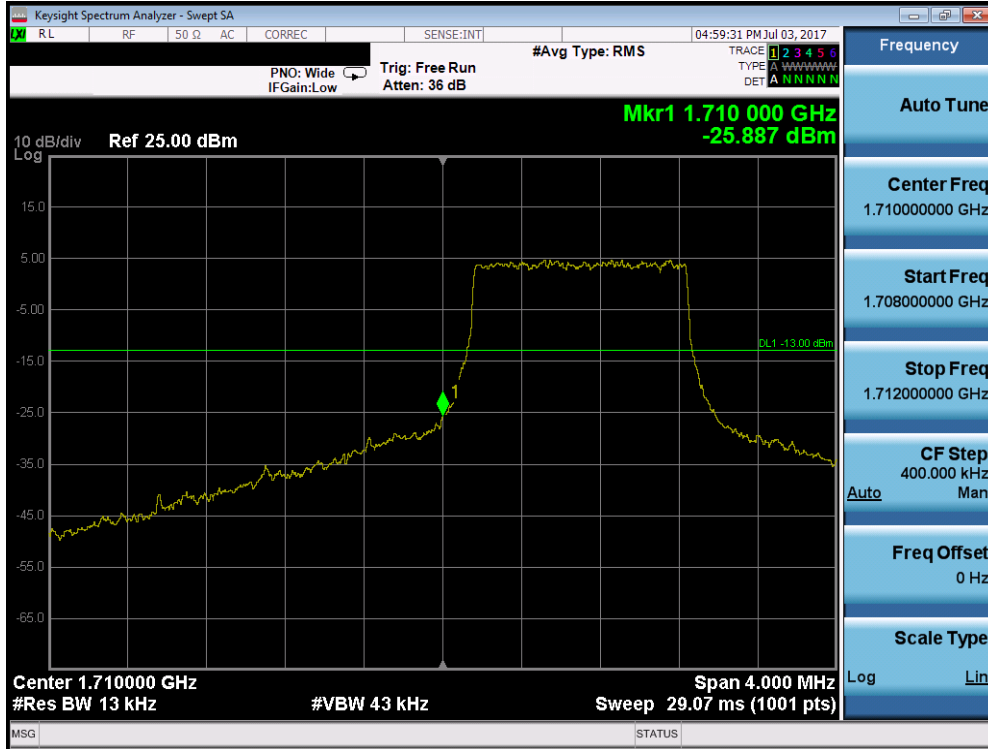
Plot 7-129. Lower Band Edge Plot (Band 66 – 1.4MHz QPSK – RB Size 6)
