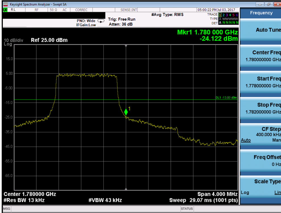
Plot 7-131. Upper Band Edge Plot (Band 66 – 1.4MHz QPSK – RB Size 6)
