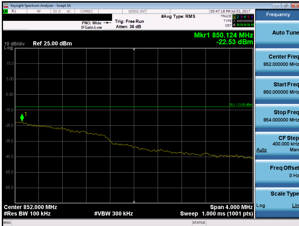
Plot 7-112. Upper Extended Band Edge Plot (Band 5 – Band 5 – 3.0MHz QPSK – RB Size 15)
