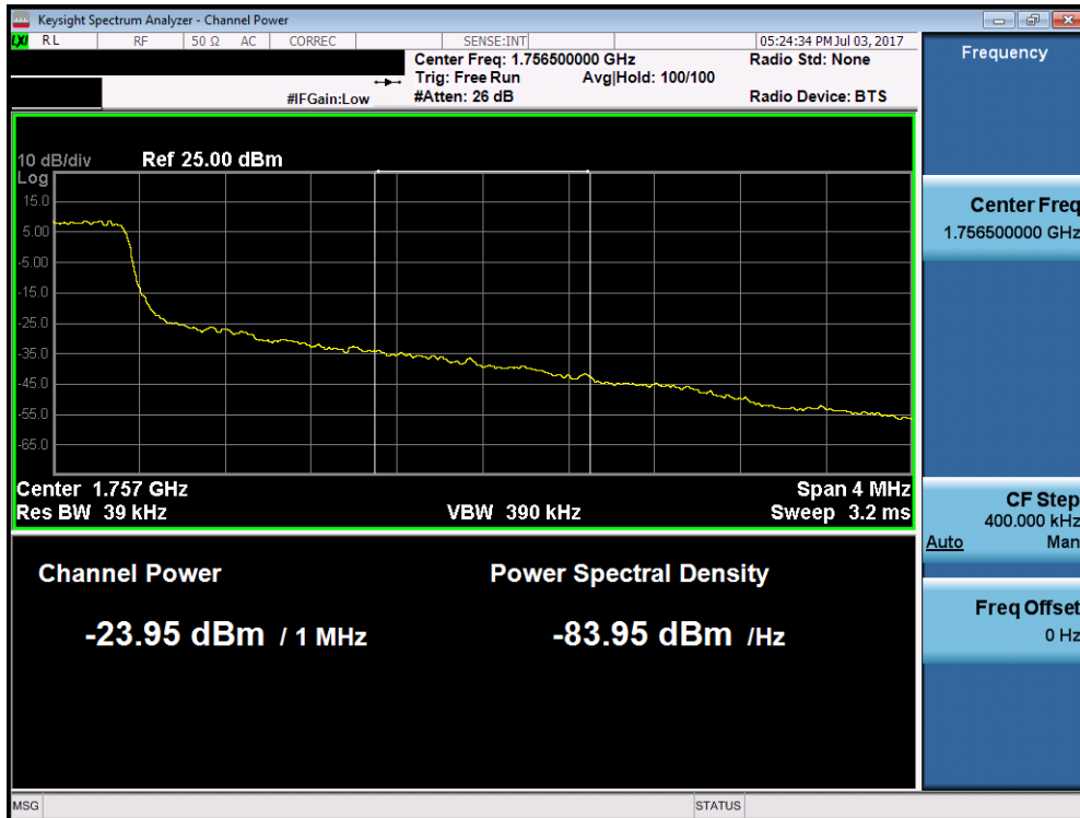
Plot 7-118. Upper Extended Band Edge Plot (Band 4 – 1.4MHz QPSK – RB Size 6)
