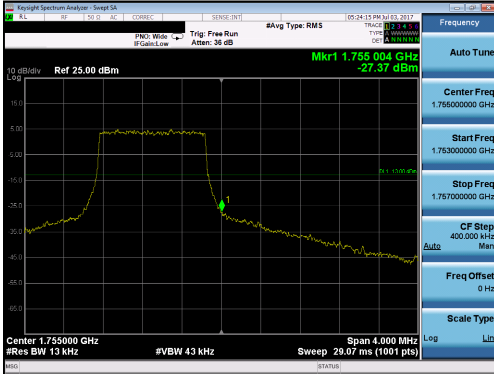
Plot 7-117. Upper Band Edge Plot (Band 4 – 1.4MHz QPSK – RB Size 6)
