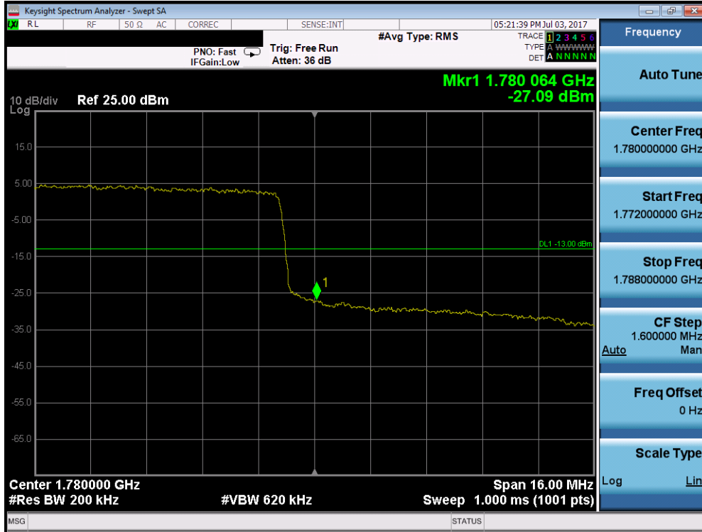
Plot 7-151. Upper Band Edge Plot (Band 66 – 20.0MHz QPSK – RB Size 100)
