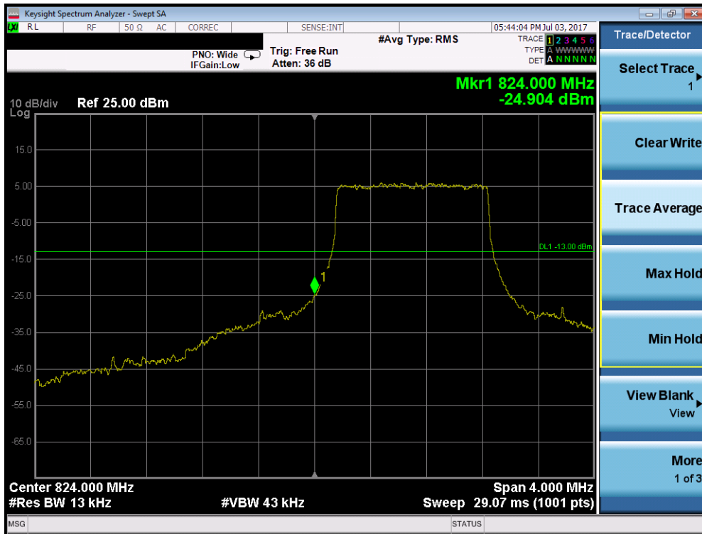
Plot 7-106. Lower Band Edge Plot (Band 5 – 1.4MHz QPSK – RB Size 6)
