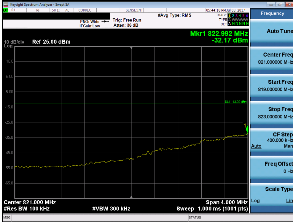
Plot 7-107. Lower Extended Band Edge Plot (Band 5 – 1.4MHz QPSK – RB Size 6)
