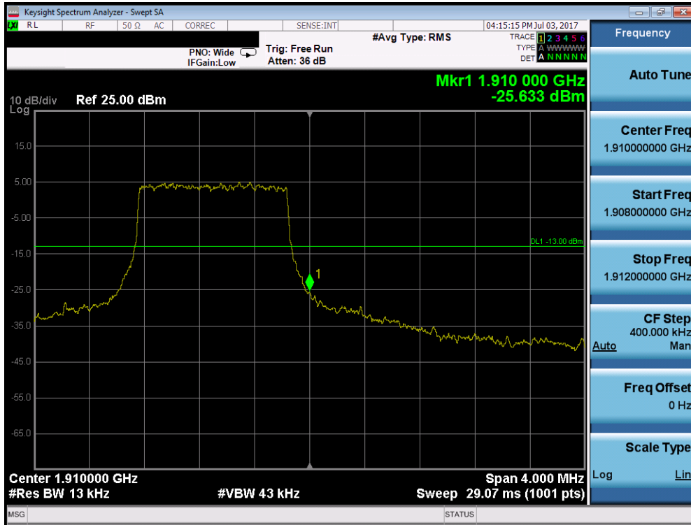
Plot 7-155. Upper Band Edge Plot (Band 2 – 1.4MHz QPSK – RB Size 6)
