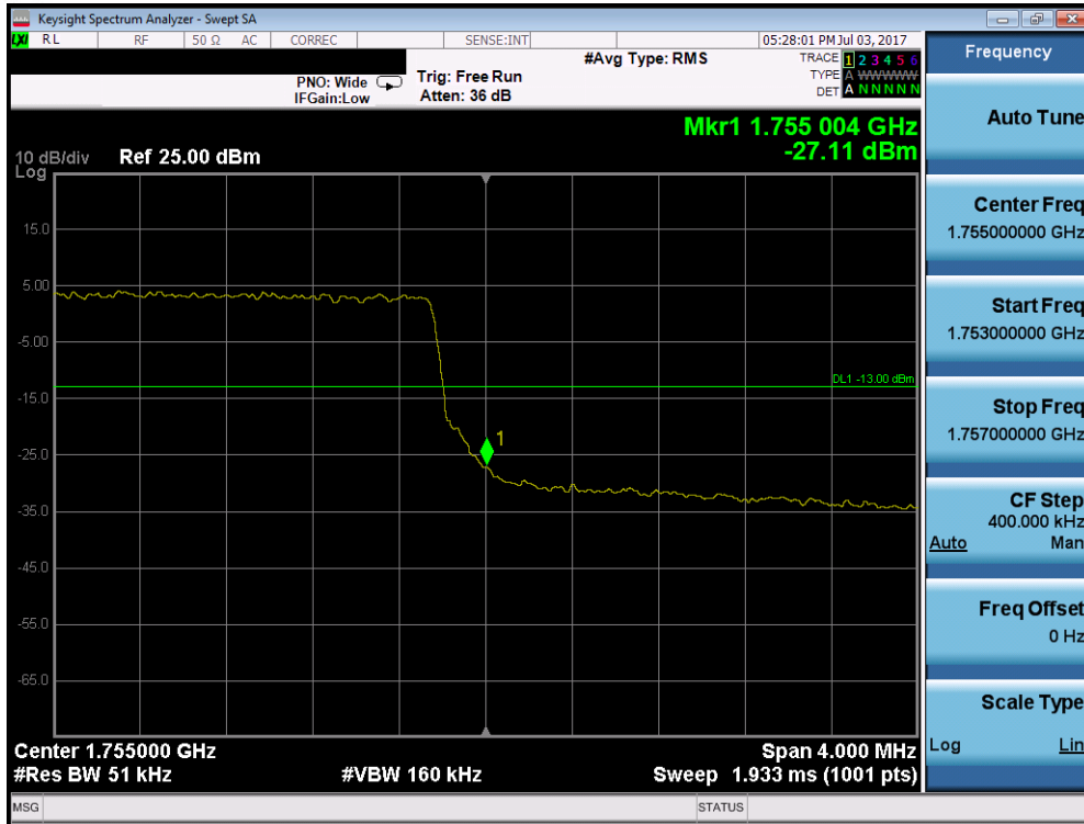
Plot 7-121. Upper Band Edge Plot (Band 4 – 5.0MHz QPSK – RB Size 25)
