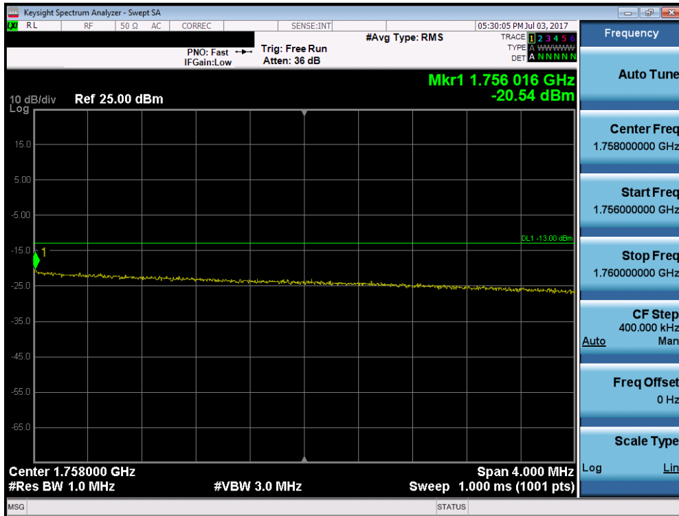
Plot 7-124. Upper Extended Band Edge Plot (Band 4 – 10.0MHz QPSK – RB Size 50)
