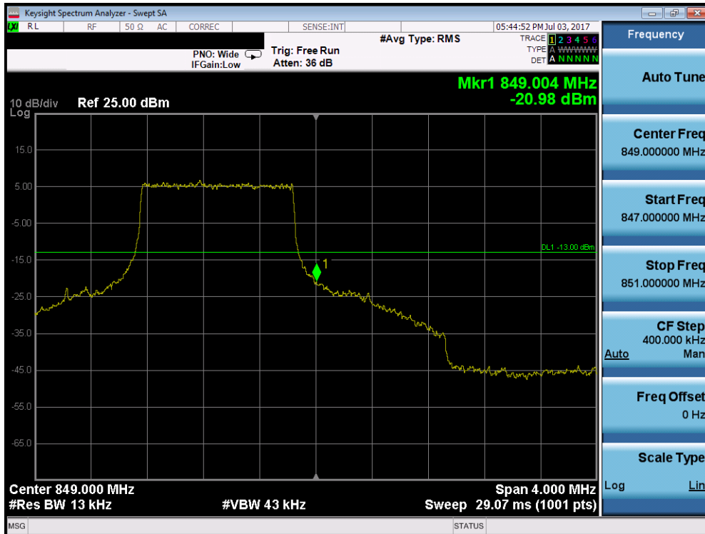
Plot 7-108. Upper Band Edge Plot (Band 5 – 1.4MHz QPSK – RB Size 6)
