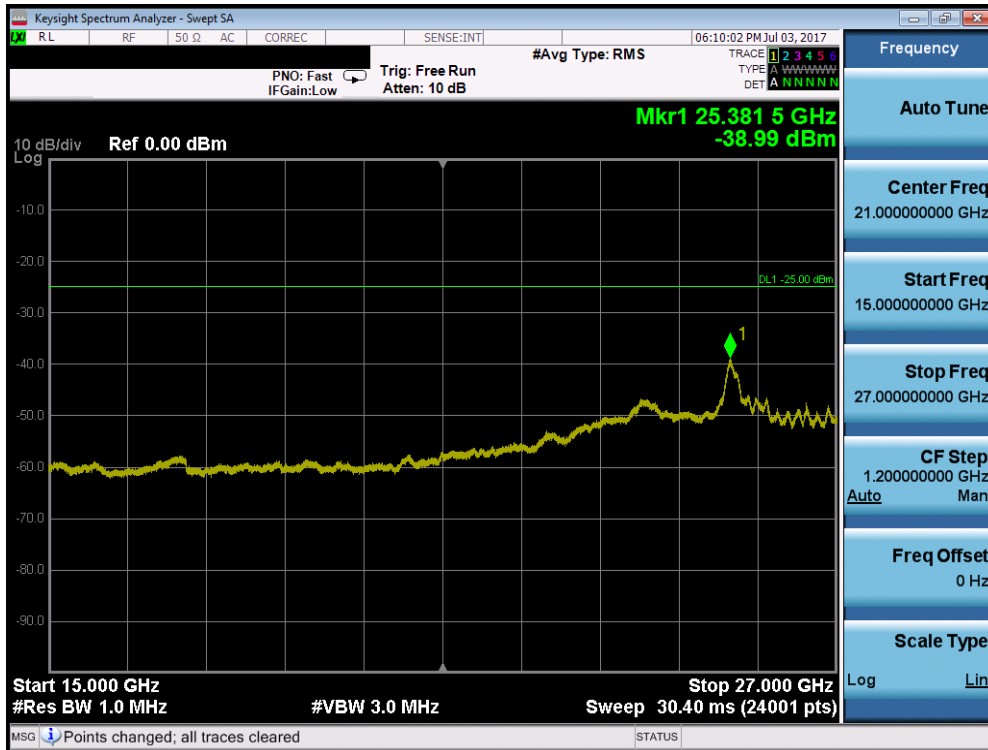
Plot 7-90. Conducted Spurious Plot (Band 7 – 15.0MHz QPSK – RB Size 1, RB Offset 0 – Mid Channel)
