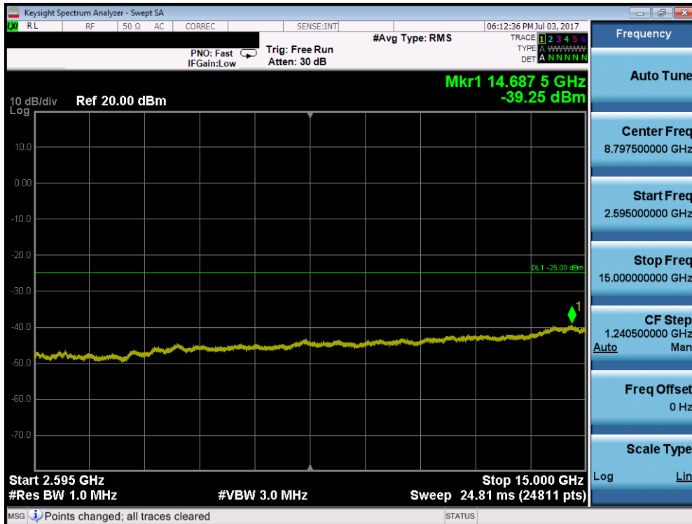
Plot 7-92. Conducted Spurious Plot (Band 7 – 15.0MHz QPSK – RB Size 1, RB Offset 0 – High Channel)
