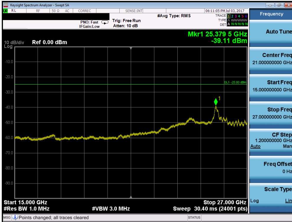
Plot 7-87. Conducted Spurious Plot (Band 7 – 15.0MHz QPSK – RB Size 1, RB Offset 0 – Low Channel)
