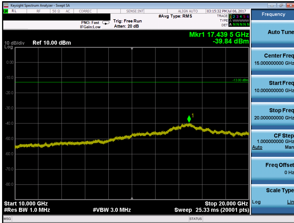
Plot 7-40. Conducted Spurious Plot (AWS WCDMA Mode – Ch. 1413)
