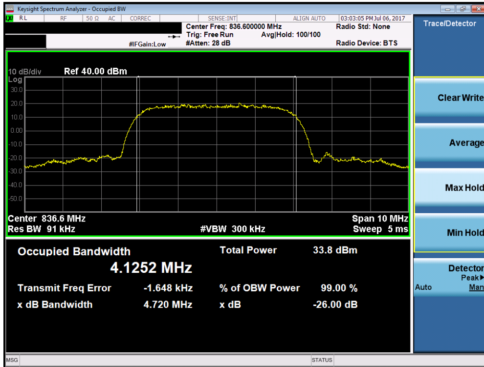
Plot 7-5. Occupied Bandwidth Plot (Cellular WCDMA Mode – Ch. 4183)
