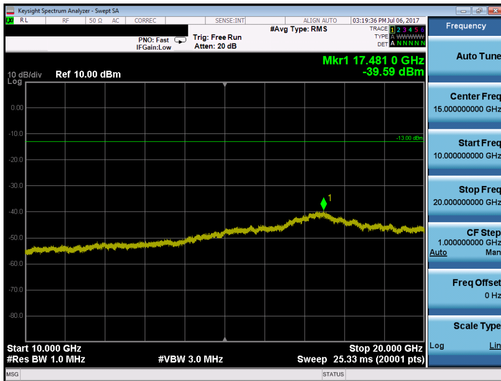
Plot 7-43. Conducted Spurious Plot (AWS WCDMA Mode – Ch. 1513)
