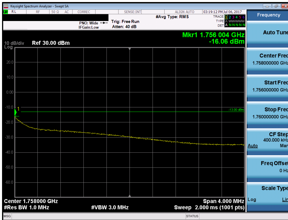
Plot 7-62. 4MHz Span Plot (AWS WCDMA Mode – Ch. 1513)
