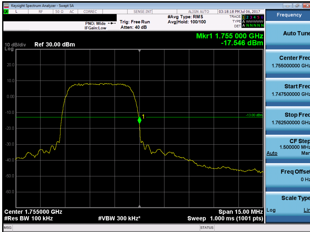
Plot 7-61. Band Edge Plot (AWS WCDMA Mode – Ch. 1513)
