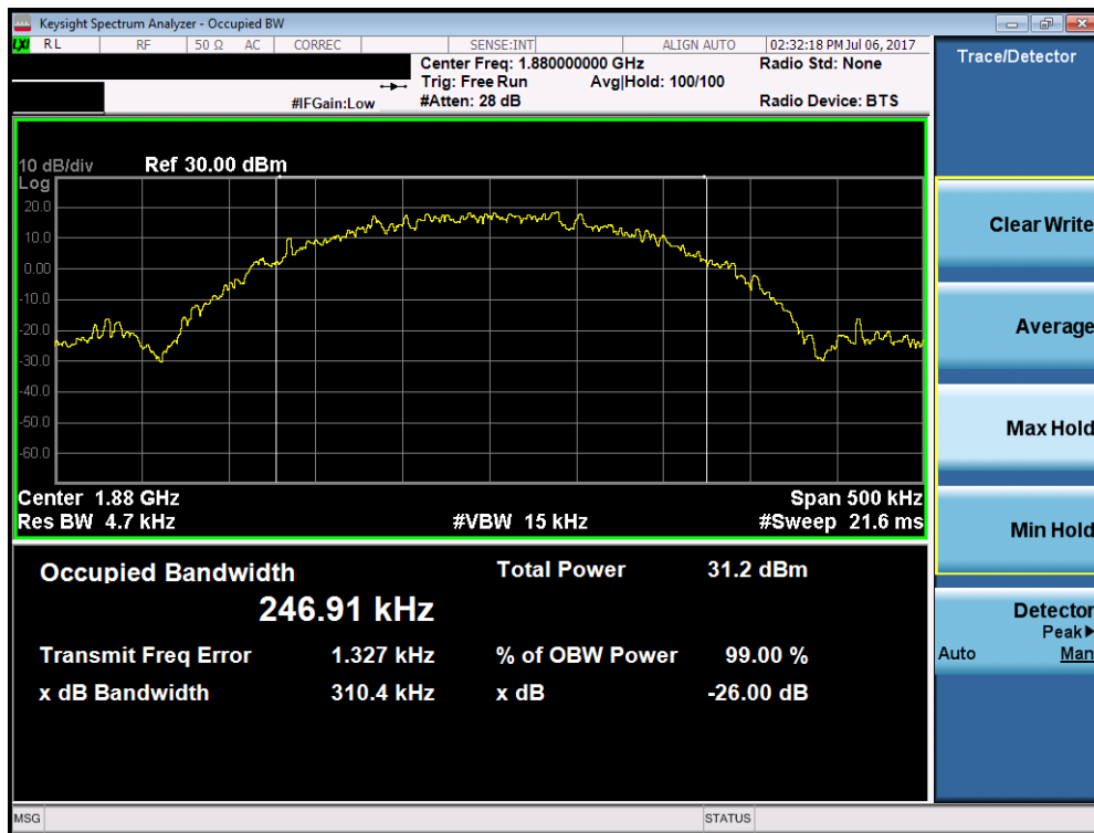
Plot 7-4. Occupied Bandwidth Plot (EDGE1900 Mode – Ch. 661)
