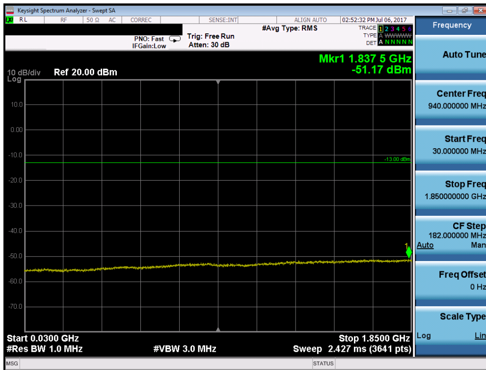
Plot 7-47. Conducted Spurious Plot (PCS WCDMA Mode – Ch. 9400)
