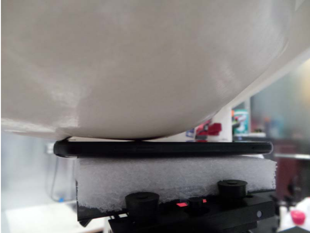
SAR Test Setup Photo 1: Right Cheek
