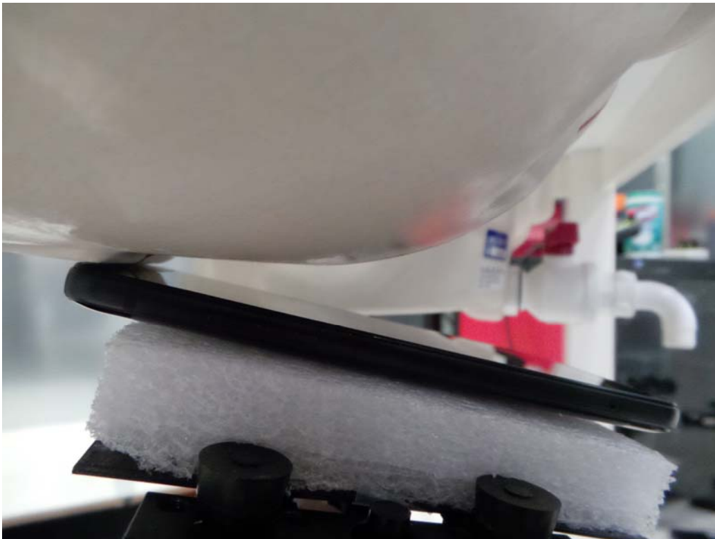
SAR Test Setup Photo 2: Right Tilt
