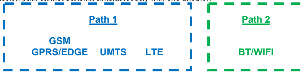
Figure 1-1 Simultaneous Transmission Paths
