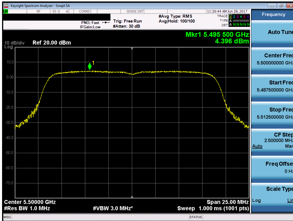
Plot 7-59. Power Spectral Density Plot (20MHz BW 802.11n (UNII Band 2C) – Ch. 100)
