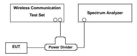
(Configuration of conducted Emission measurement)
