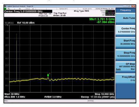
BAND 17. Conducted Spurious Plot\_ (23780ch\_10MHz\_QPSK\_RB 1\_0)
