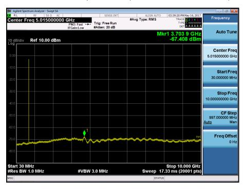
BAND 17. Conducted Spurious Plot\_ (23790ch\_5MHz\_QPSK\_RB 1\_0)
