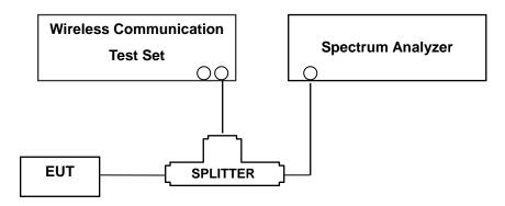
(Configuration of conducted Emission measurement)
