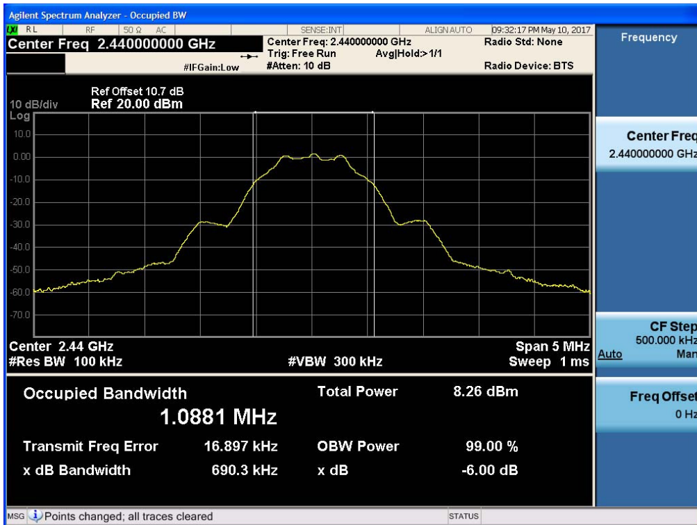
6 dB Bandwidth plot (Mid-CH 19)
