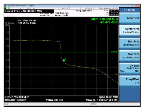
BAND 17. Upper Band Edge Plot (10M BW Ch.23800 QPSK\_RB50) -2
