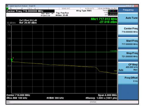
BAND 17. Upper Extended Band Edge Plot (5M BW Ch.23825 QPSK\_RB25) -3
