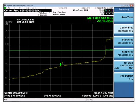
BAND 17. Lower Band Edge Plot (10M BW Ch.23780 QPSK RB 50) -2
