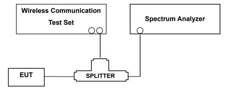
(Configuration of conducted Emission measurement)
