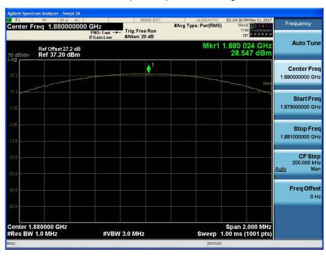
■ GSM1900 EDGE (661 CH.) Peak-to-Average Ratio P<sub>Avq</sub>
