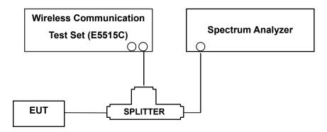
(Configuration of conducted Emission measurement)
