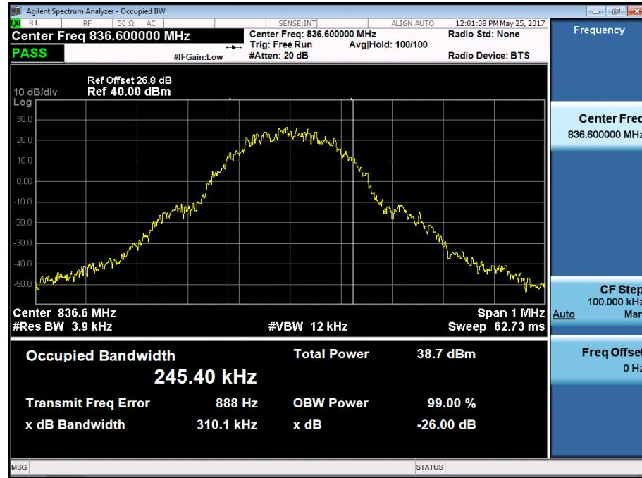
■ GSM850 MODE (251 CH.) Occupied Bandwidth
