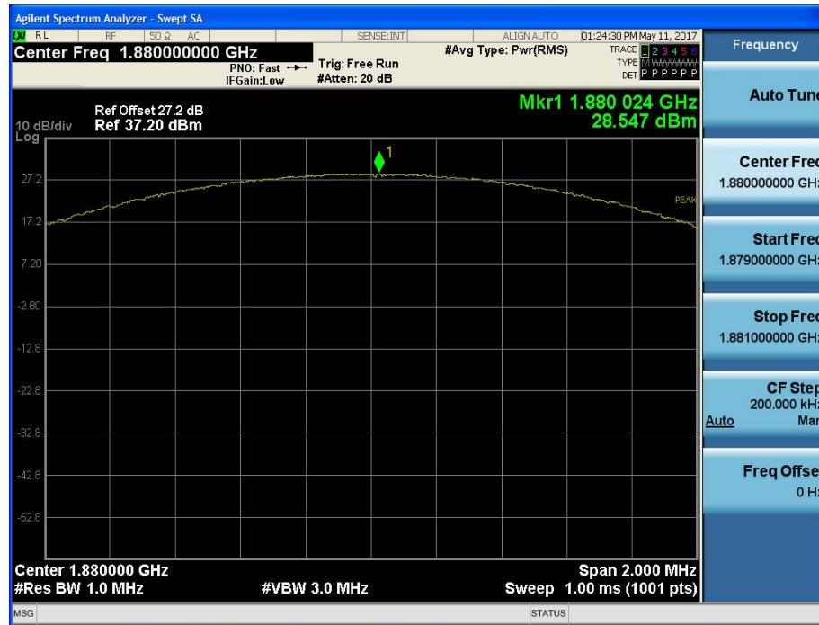
■ GSM1900 EDGE (661 CH.) Peak-to-Average Ratio P<sub>Avg</sub>
