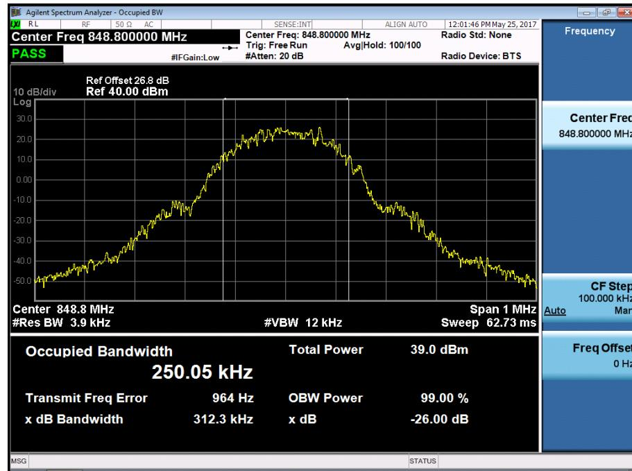
■ GSM850 EDGE (251 CH.) Occupied Bandwidth
