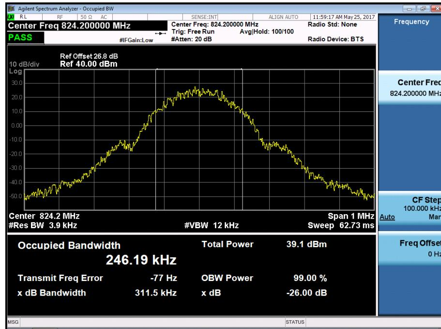
■ GSM850 MODE (190 CH.) Occupied Bandwidth
