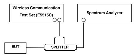
(Configuration of conducted Emission measurement)
