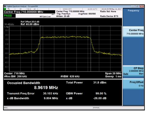
BAND 17. Occupied Bandwidth Plot (10M BW Ch.23790 16QAMRB 50)
