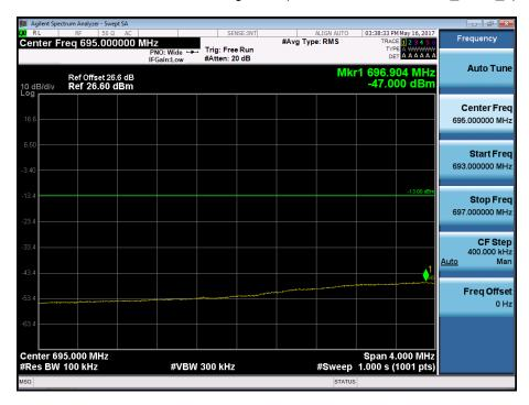
BAND 17. Lower Band Edge Plot (10M BW Ch.23780 QPSK RB 1, Offset 0) -1
