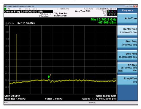
BAND 17. Conducted Spurious Plot\_ (23790ch\_5MHz\_QPSK\_RB 1\_0)
