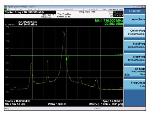
BAND 17. Upper Band Edge Plot (5M BW Ch.23825 QPSK\_RB25) -2
