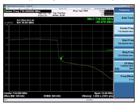
BAND 17. Upper Extended Band Edge Plot (10M BW Ch.23800 QPSK\_RB50) -3
