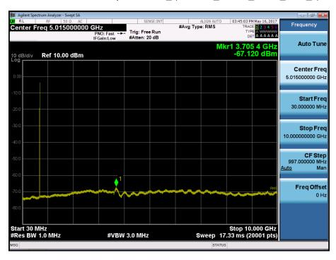
BAND 17. Conducted Spurious Plot\_ (23800ch\_10MHz\_QPSK\_RB 1\_0)
