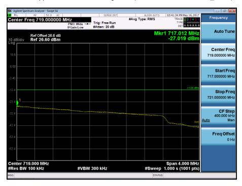
BAND 17. Upper Band Edge Plot (10M BW Ch.23800 QPSK\_RB1\_Offset 49) -1
