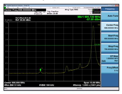
BAND 17. Lower Band Edge Plot (5M BW Ch.23755 QPSK RB 25) -2
