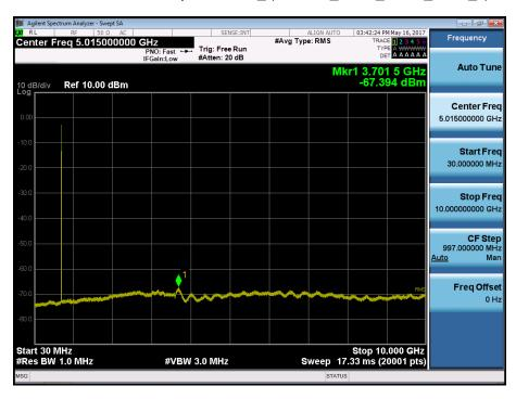
BAND 17. Conducted Spurious Plot\_ (23780ch\_10MHz\_QPSK\_RB 1\_0)
