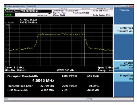
BAND 17. Occupied Bandwidth Plot (5M BW Ch.23790 16QAM RB 25)
