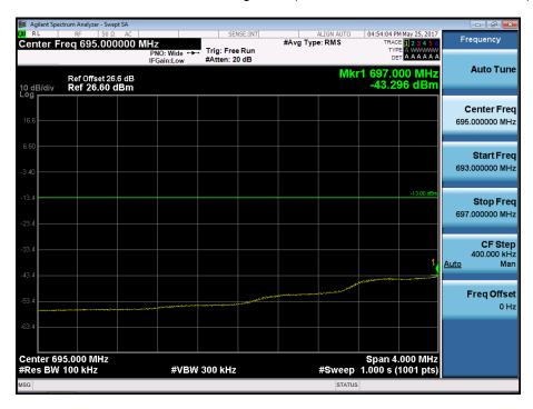
BAND 12. Lower Band Edge Plot (3M BW Ch.23025 QPSK\_RB1\_Offset 0)
