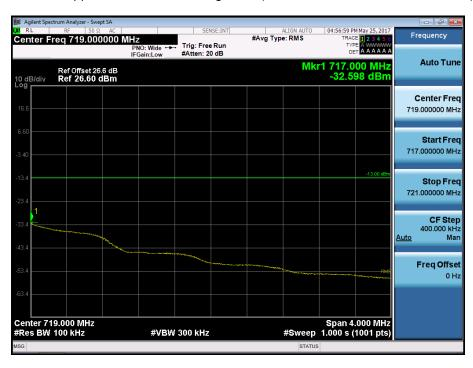
BAND 12. Upper Band Edge Plot (3M BW Ch.23165 QPSK\_RB1\_Offset 14)
