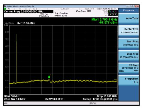
BAND 12. Conducted Spurious Plot \_ (23060ch\_10MHz\_QPSK\_RB 1\_0)
