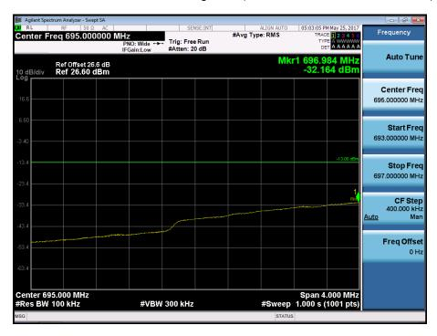
BAND 12. Lower Band Edge Plot (10M BW Ch.23060 QPSK\_RB1\_Offset 0)
