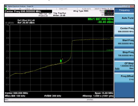
BAND 12. Lower Extended Band Edge Plot (10M BW Ch.23060 QPSK\_RB50\_0)
