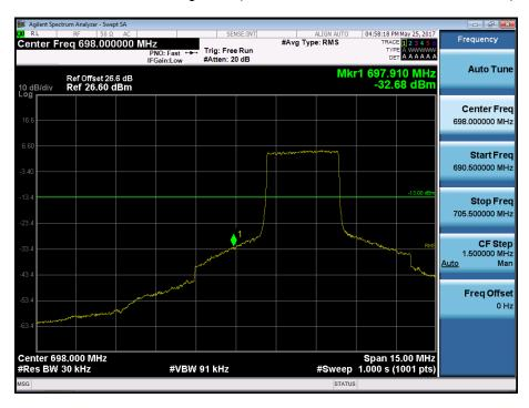
BAND 12. Lower Extended Band Edge Plot (3M BW Ch.23025 QPSK\_RB15\_0)
