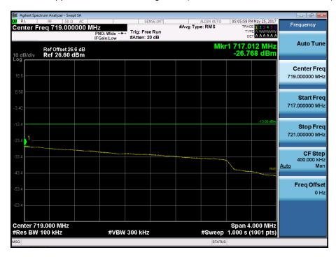
BAND 12. Upper Band Edge Plot (10M BW Ch.23130 QPSK\_RB1\_Offset 49)
