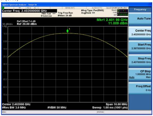
Test Plots ( $\pi/4DQPSK$ ) Peak Power (CH.39)
