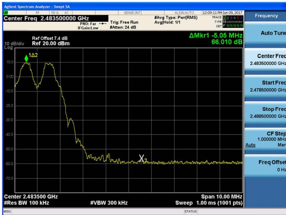
Test Plots with hopping (8DPSK)
