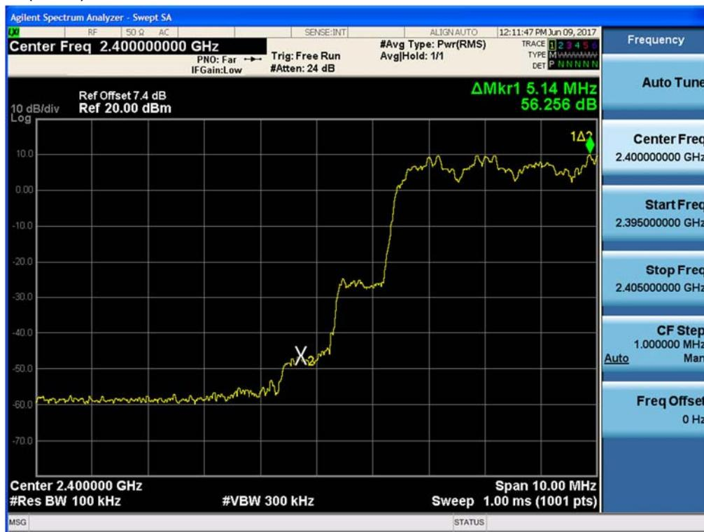
Test Plots with hopping (8DPSK)
