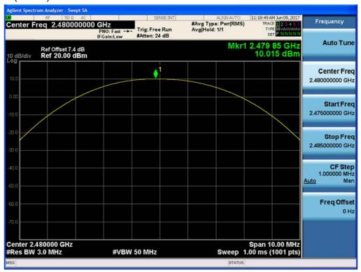
Test Plots (8DPSK) Peak Power (CH.0)
