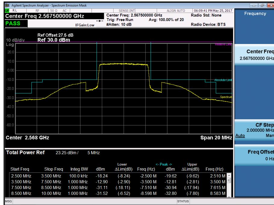
BAND 7. Low Channel Edge Plot (10MHz Ch.20800 QPSK\_RB50\_0)
