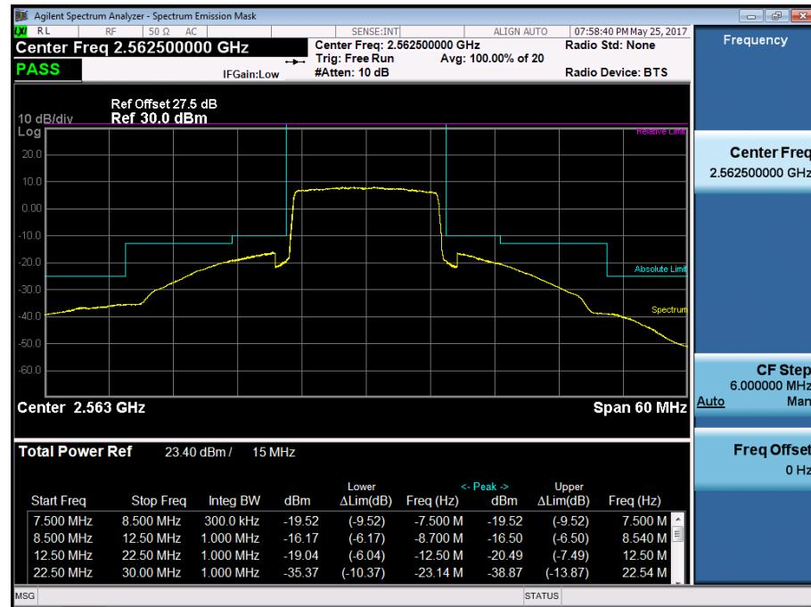
BAND 7. Low Channel Edge Plot (20MHz Ch.20850 QPSK\_RB100\_0)-1
