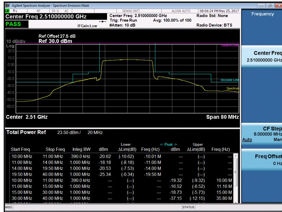
BAND 7. Low Channel Edge Plot (20MHz Ch.20850 QPSK\_RB100\_0)-2
