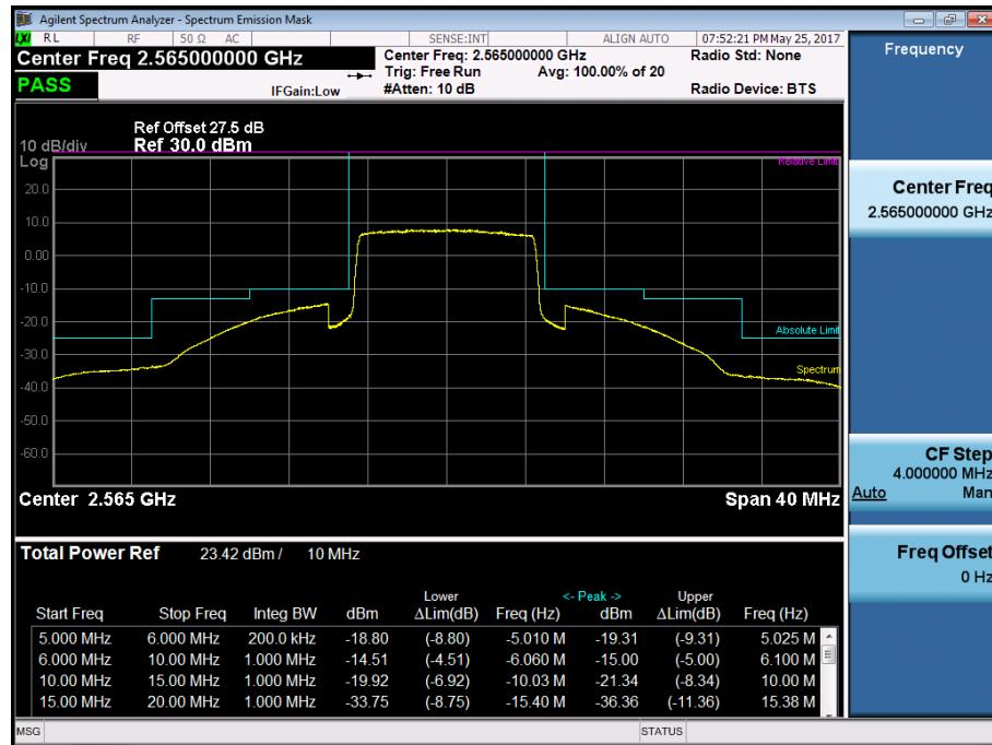
BAND 7. Low Channel Edge Plot (15MHz Ch.20825 QPSK\_RB75\_0)
