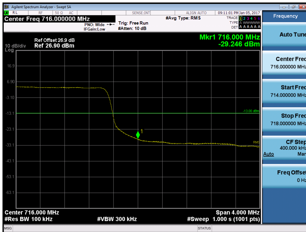
BAND 12 / 17. Upper Band Edge Plot (10M BW Ch.23130 QPSK_RB50_Offset 0)
