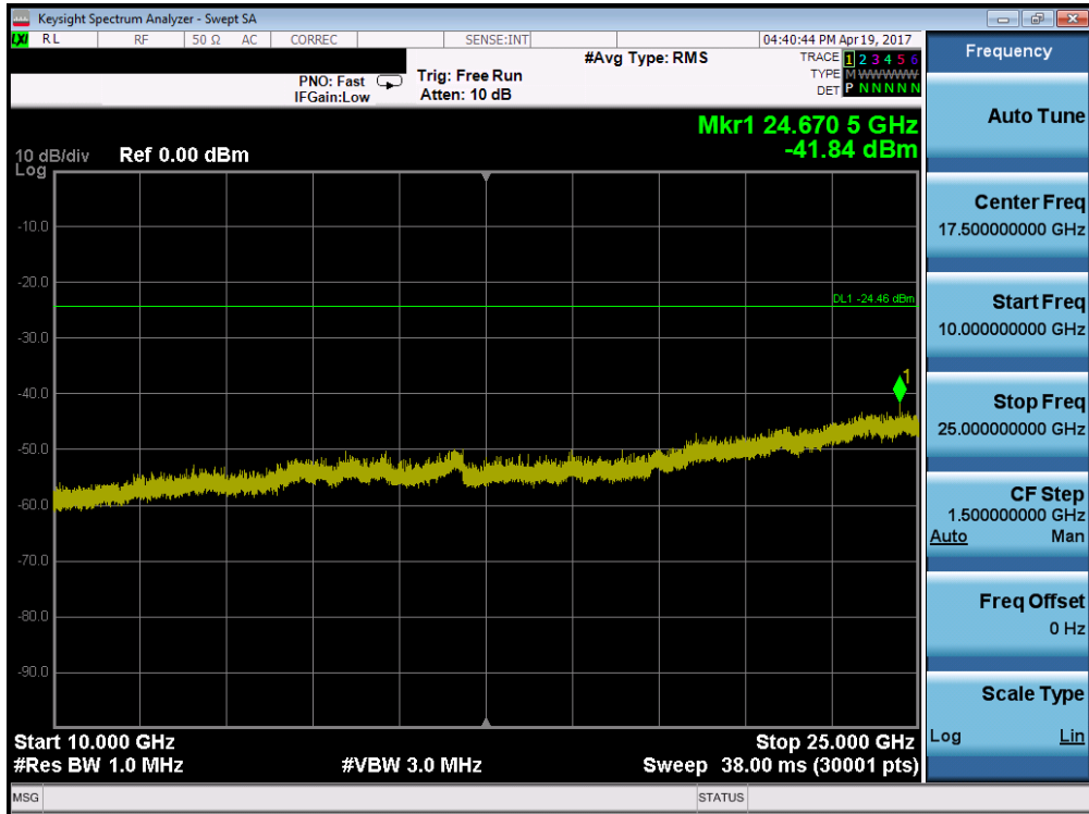
Plot 7-28. Conducted Spurious Plot (802.11b – Ch. 6)
