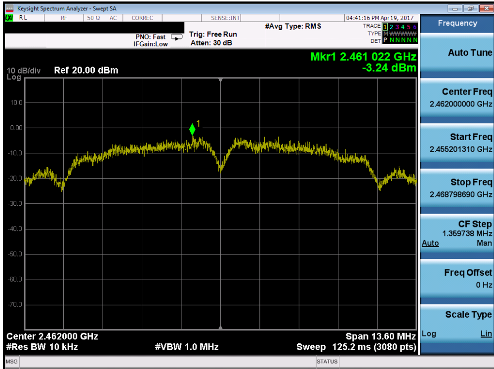
Plot 7-12. Power Spectral Density Plot (802.11b – Ch. 11)
