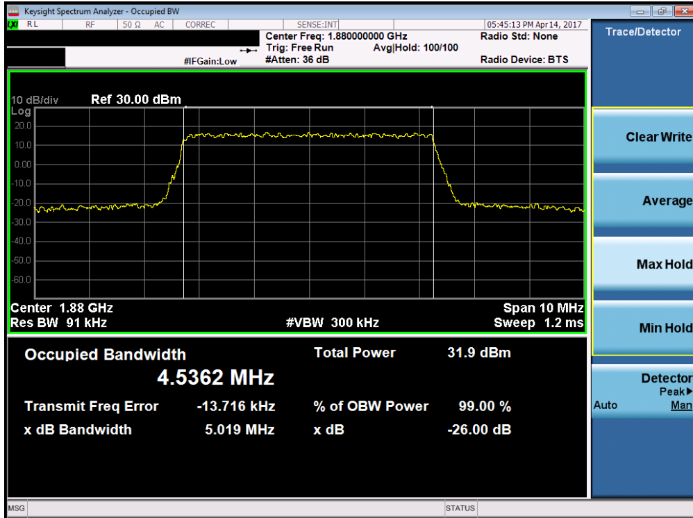
Plot 7-29. Occupied Bandwidth Plot (Band 2 – 5.0MHz QPSK – RB Size 25)
