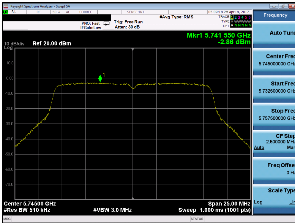
Plot 7-59. Power Spectral Density Plot (802.11a (UNII Band 3) – Ch. 149)
