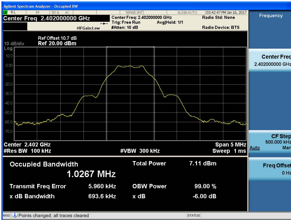
6 dB Bandwidth plot (Low-CH 0)
