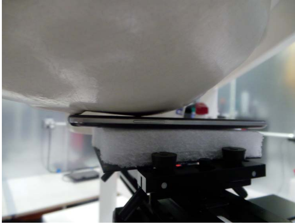
SAR Test Setup Photo 1: Right Cheek
