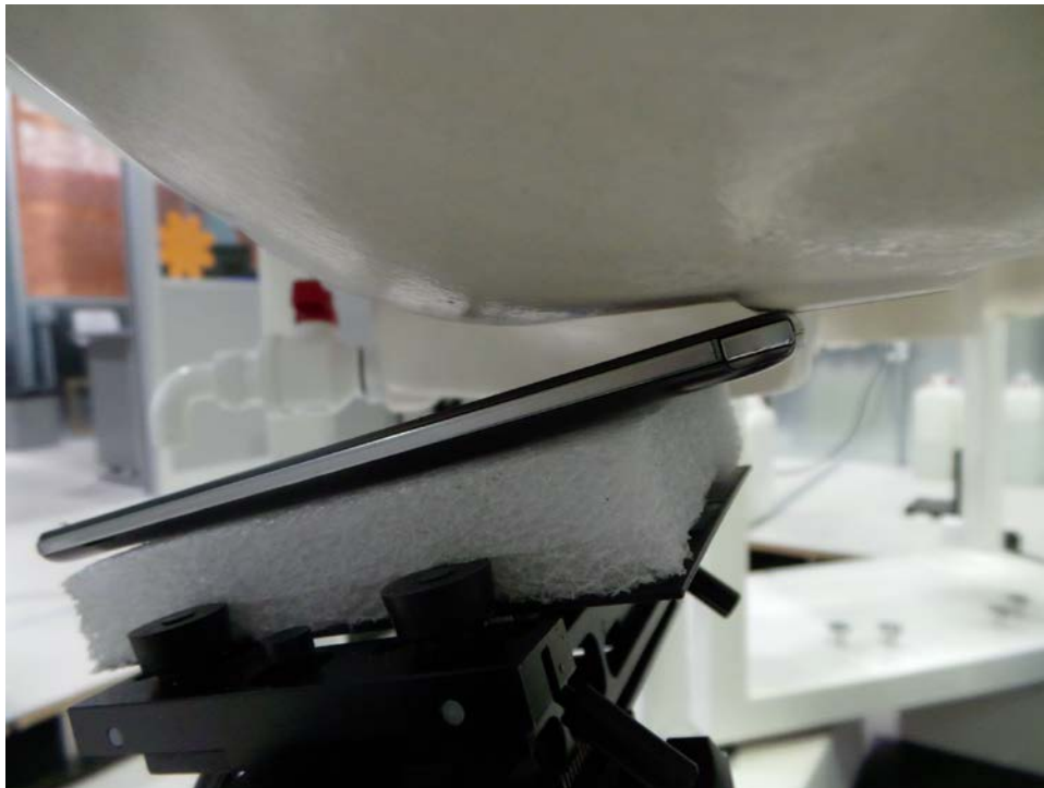
SAR Test Setup Photo 4: Left Tilt
