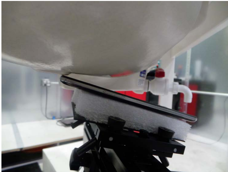
SAR Test Setup Photo 2: Right Tilt
