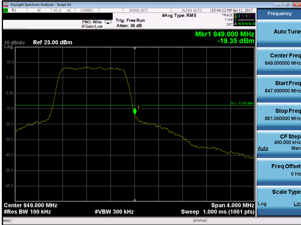
Plot 7-118. Upper Band Edge Plot (Band 5 – 1.4MHz QPSK – RB Size 6)
