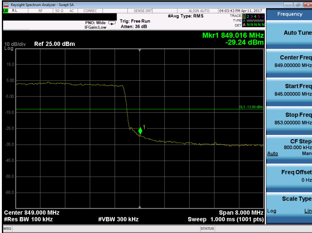
Plot 7-124. Upper Band Edge Plot (Band 5 – 10.0MHz QPSK – RB Size 50)
