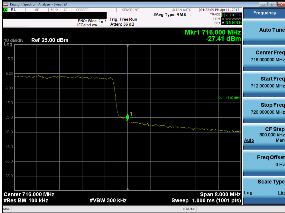
Plot 7-108. Upper Band Edge Plot (Band 12/17 – 10.0MHz QPSK – RB Size 50)
