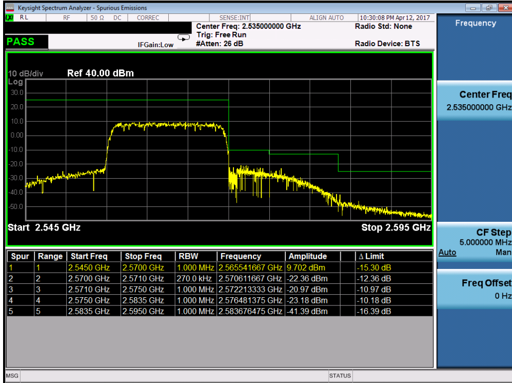
Plot 7-178. Upper ACP Plot (Band 7 – 15.0MHz QPSK – RB Size 75)
