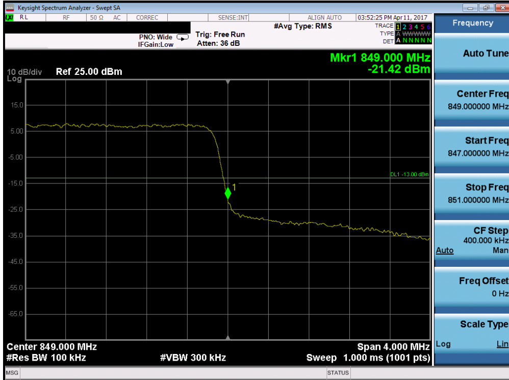
Plot 7-120. Upper Band Edge Plot (Band 5 – 3.0MHz QPSK – RB Size 15)
