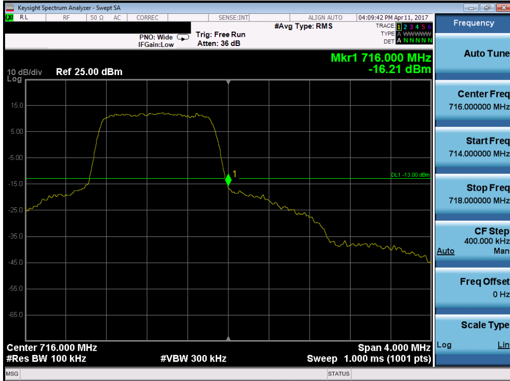
Plot 7-102. Upper Band Edge Plot (Band 12 – 1.4MHz QPSK – RB Size 6)
