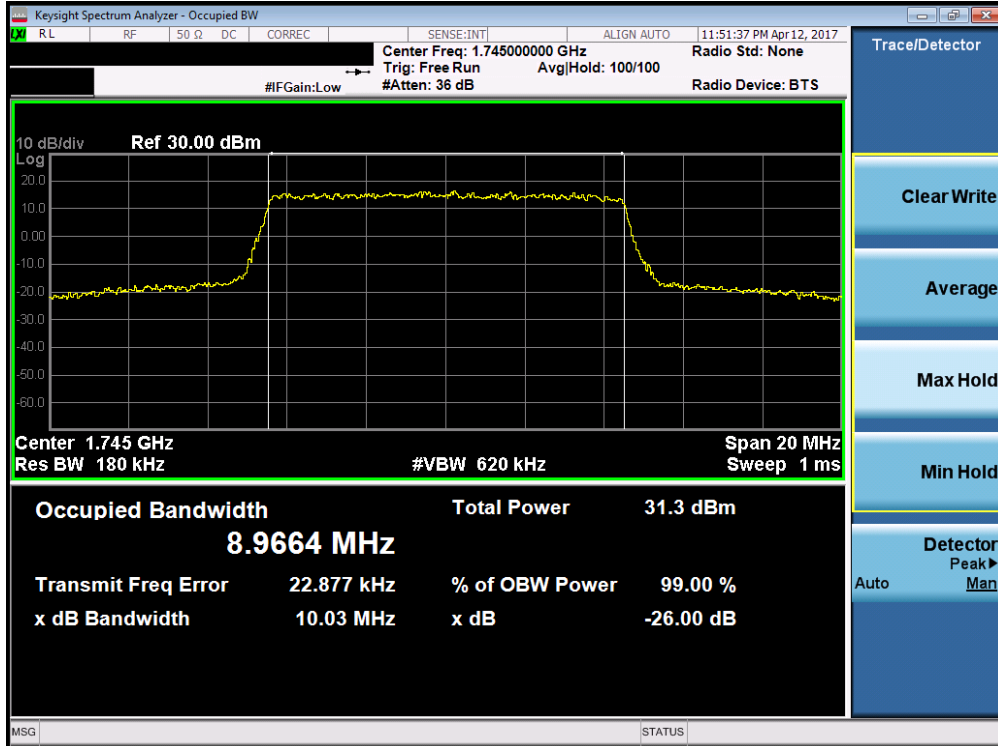
Plot 7-27. Occupied Bandwidth Plot (Band 4/66 – 10.0MHz QPSK – RB Size 50)
