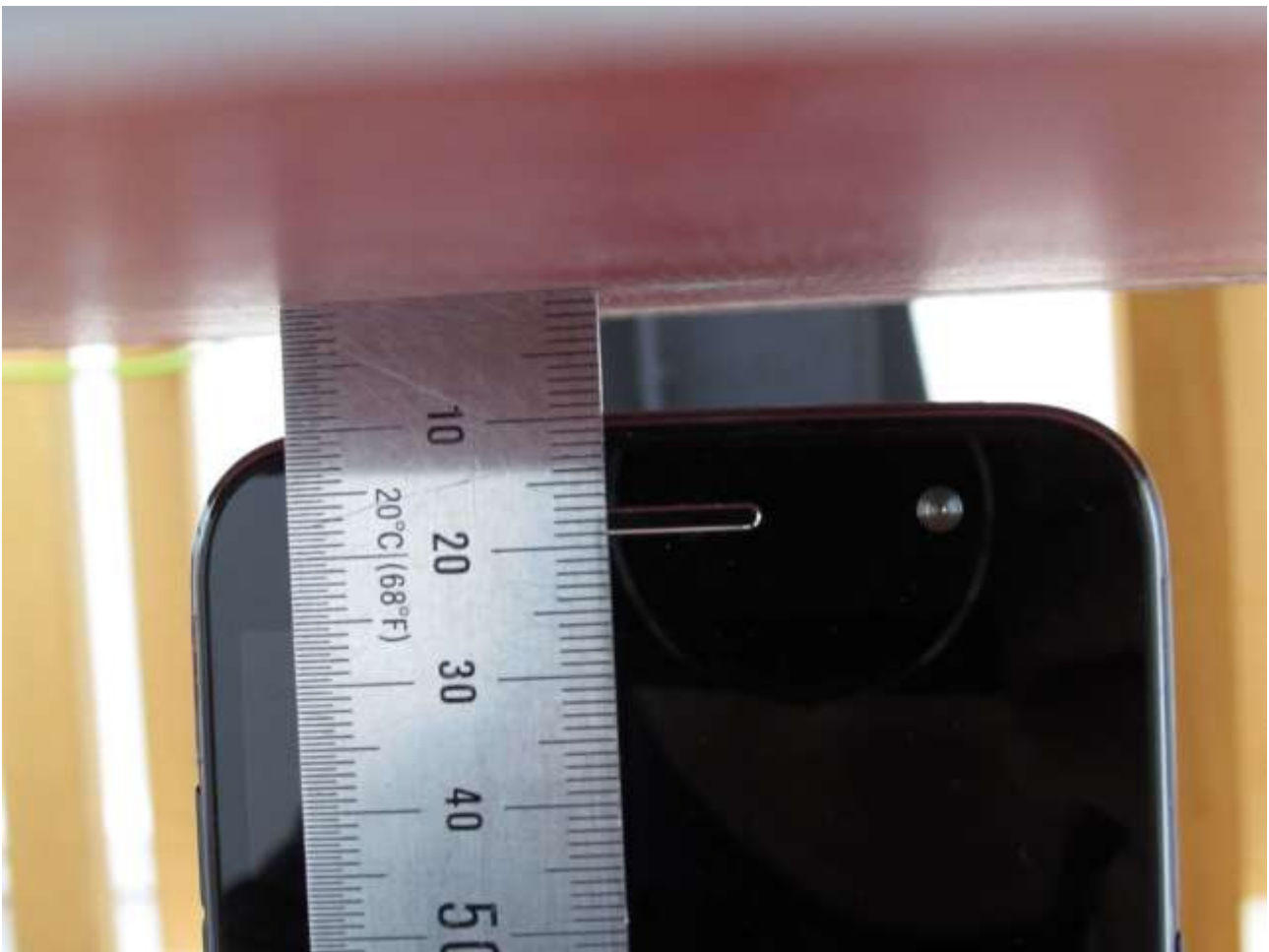
[Distance of 1.0 cm from the EUT]
