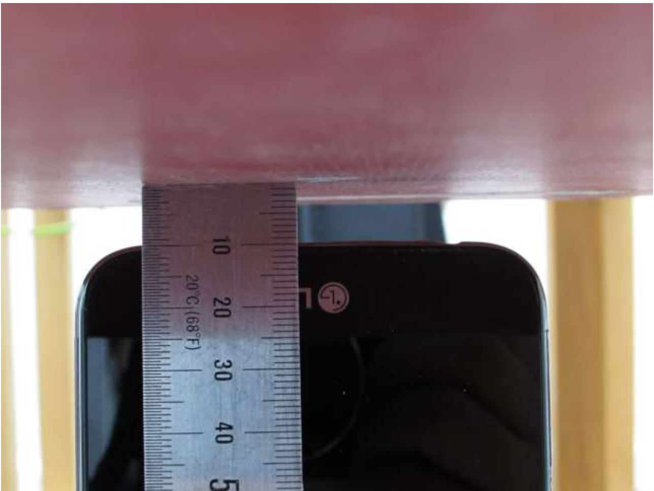
[Distance of 1.0 cm from the EUT]
