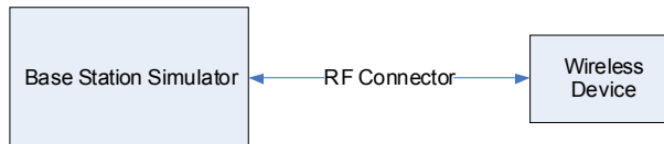
Figure 9-1 Power Measurement Setup
