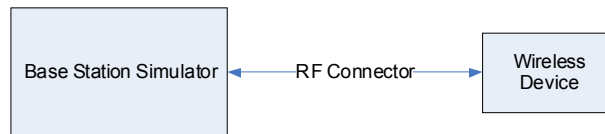
Figure 9-2 Power Measurement Setup
