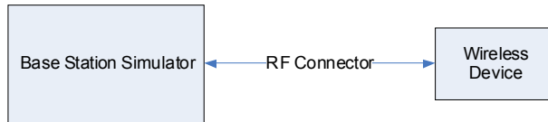
Figure 9-3 Power Measurement Setup
