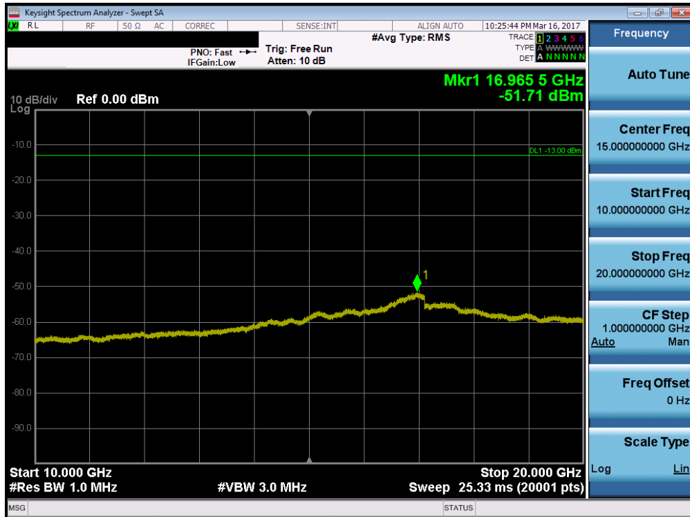
Plot 7-76. Conducted Spurious Plot (Band 2 – 20.0MHz QPSK – RB Size 1, RB Offset 0 – High Channel)
