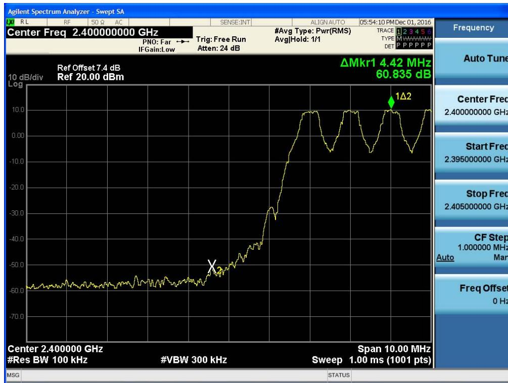
Test Plots with hopping (GFSK)
