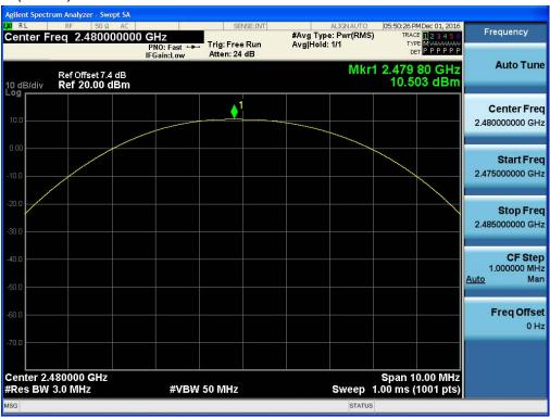
Test Plots (8DPSK) Peak Power (CH.0)
