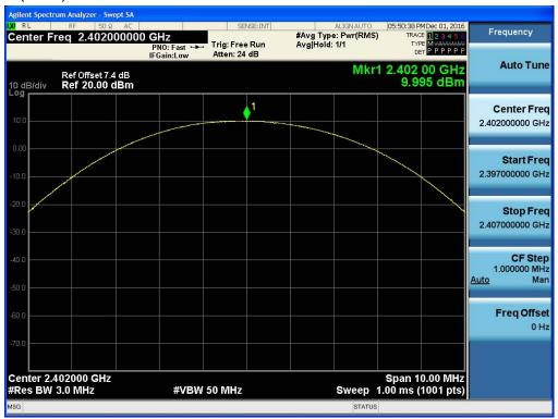
Test Plots (π/4DQPSK) Peak Power (CH.39)
