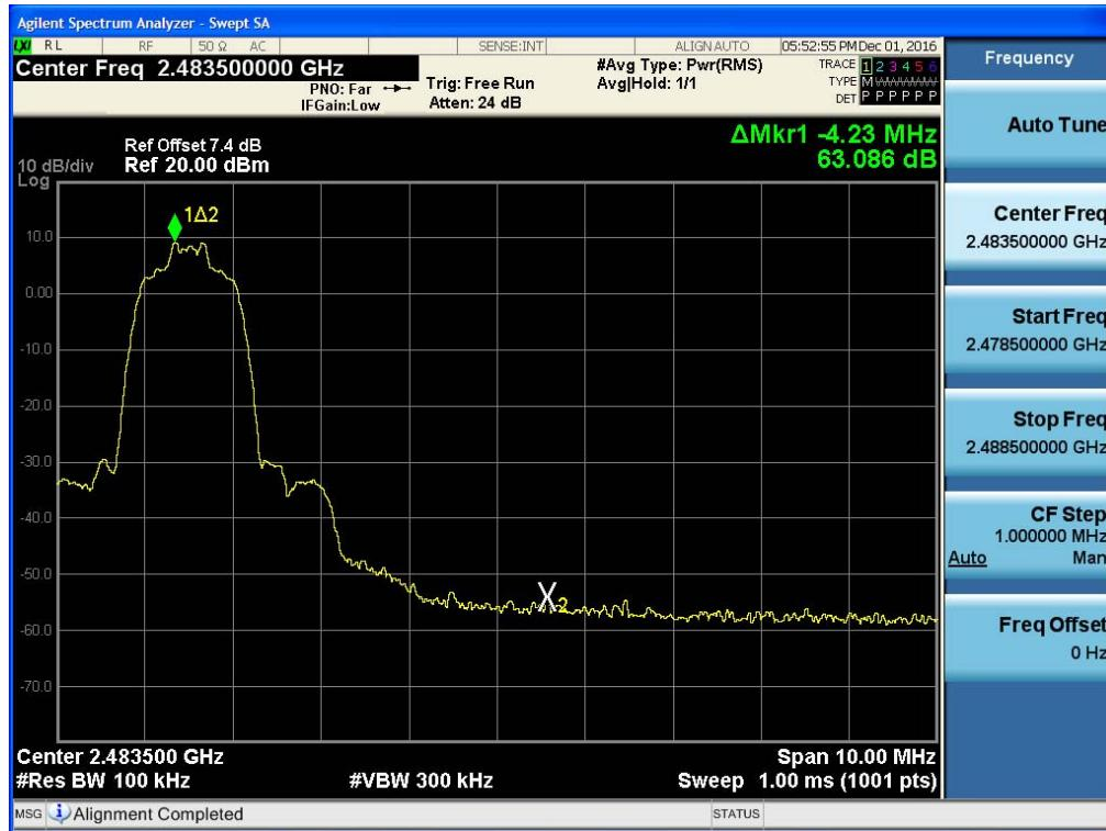
Test Plots with hopping (GFSK)
