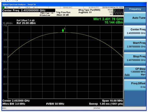
Test Plots (GFSK) Peak Power (CH.39)
