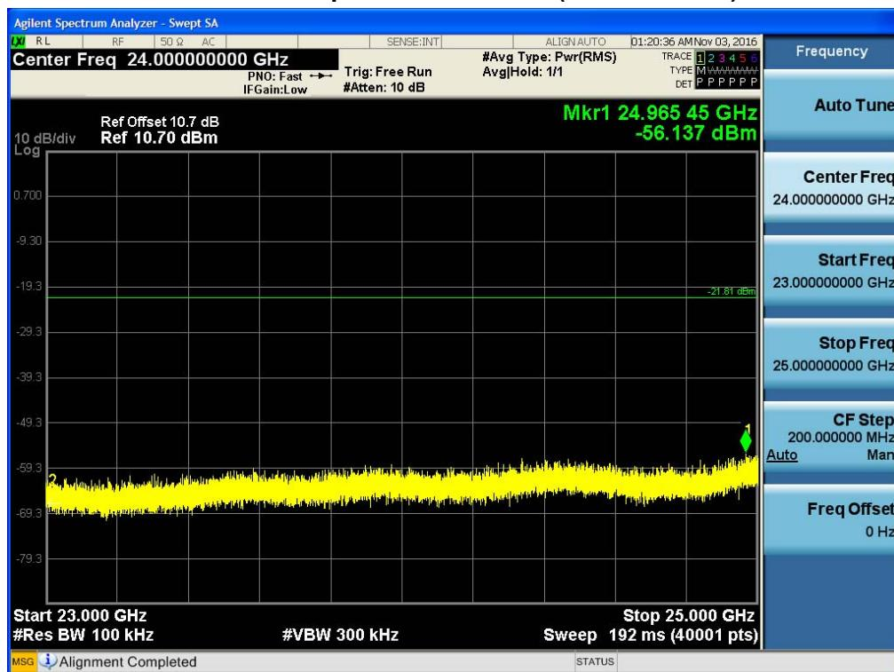
**9.6 RADIATED MEASUREMENT.****9.6.1 RADIATED SPURIOUS EMISSIONS.****Test Requirements and limit, §15.205, §15.209**
