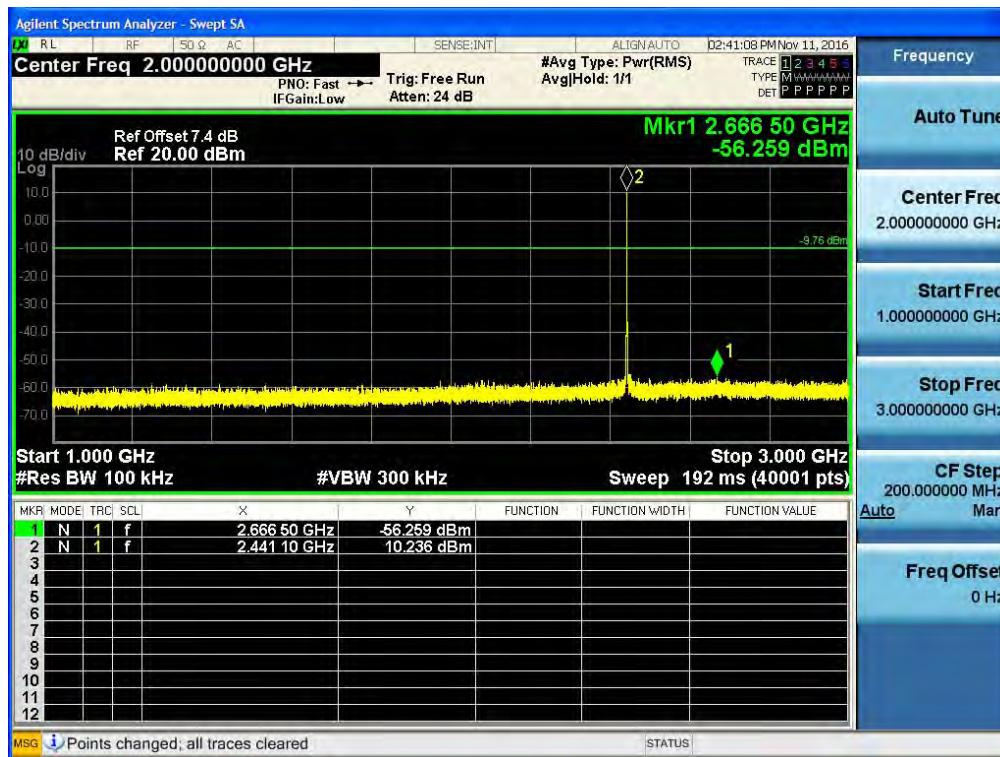
Test Plots(GFSK)- 3 GHz - 5 GHz
