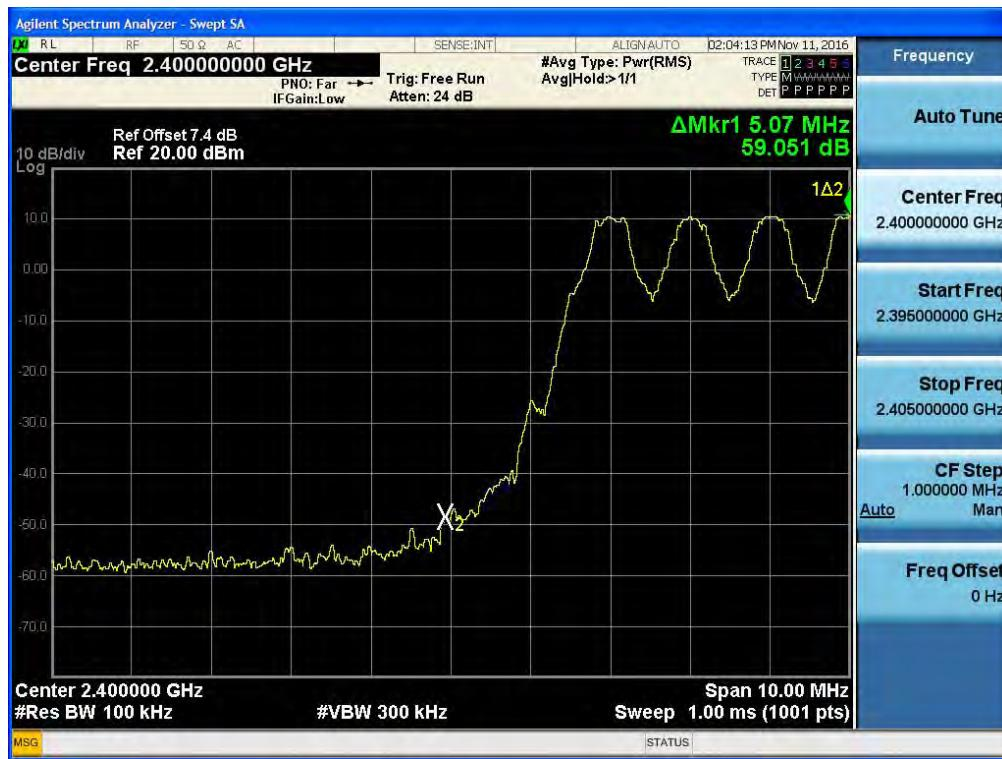
Test Plots with hopping (GFSK)
