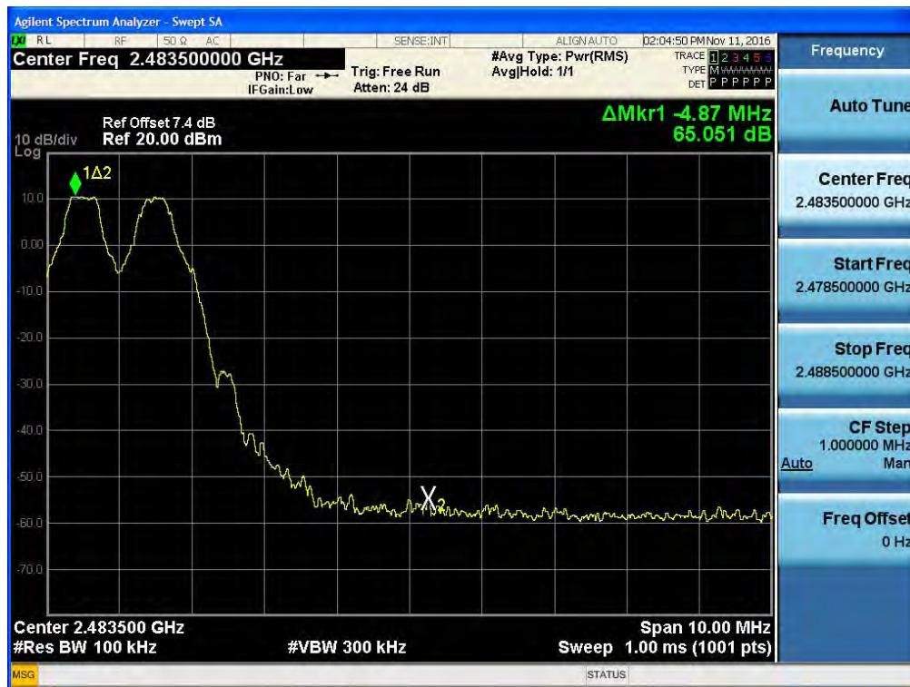
Test Plots with hopping (8DPSK)
