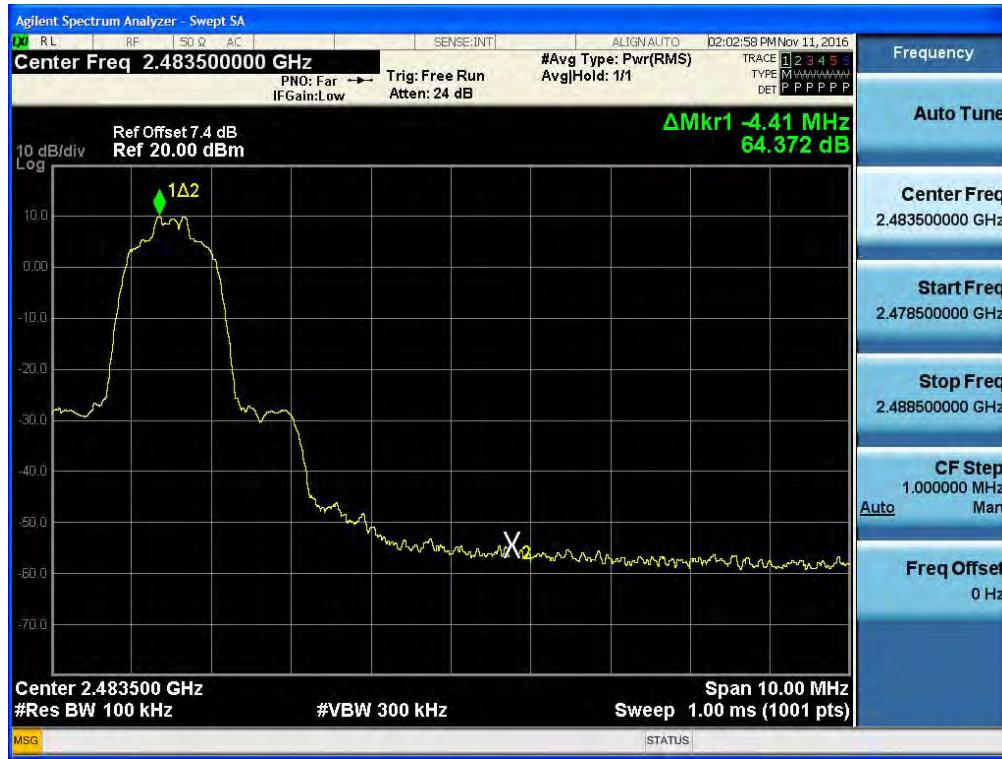
Test Plots with hopping (GFSK)
