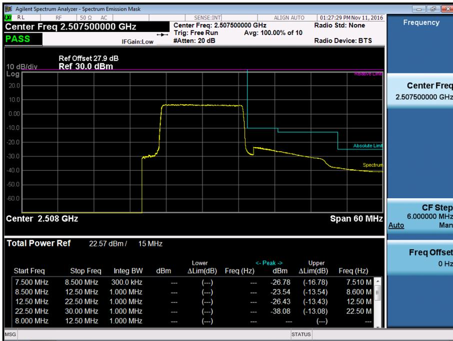
BAND7. Mid Channel Edge Plot (15MHz Ch.21100 QPSK RB 75)
