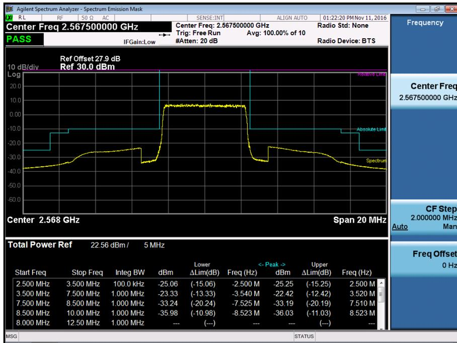
BAND7. Low Channel Edge Plot (10MHz Ch.20800 QPSK RB 50)-1
