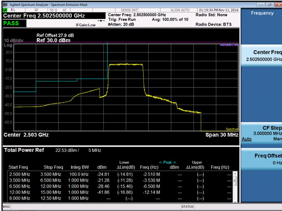
BAND7. Low Channel Edge Plot (5MHz Ch.20775 QPSK RB 25)-2
