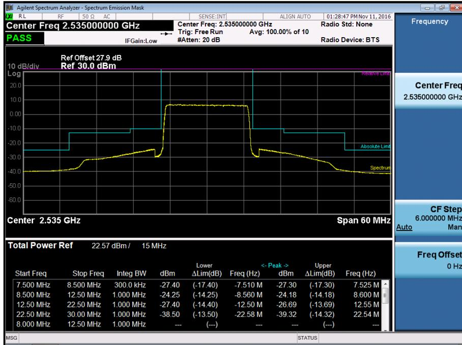
BAND7. High Channel Edge Plot (15MHz Ch.21375 QPSK RB 75)
