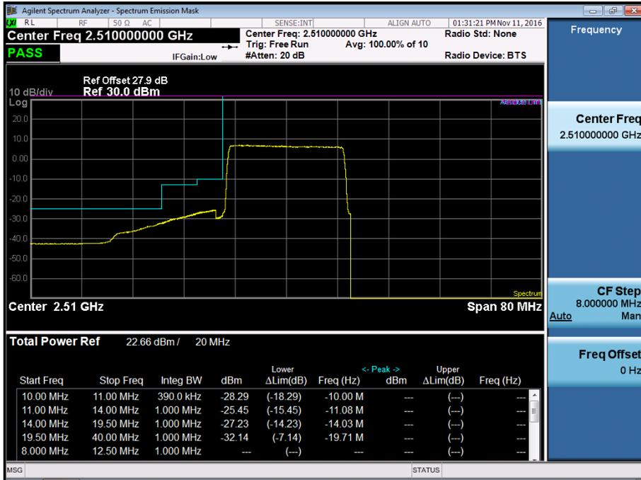
BAND7. Low Channel Edge Plot (20MHz Ch.20850 QPSK RB 100)-2
