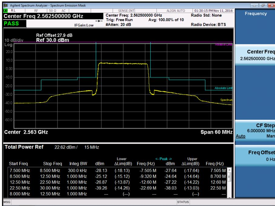
BAND7. Low Channel Edge Plot (20MHz Ch.20850 QPSK RB 100)-1
