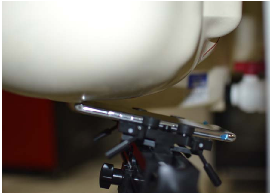
SAR Test Setup Photo 2: Right Tilt
