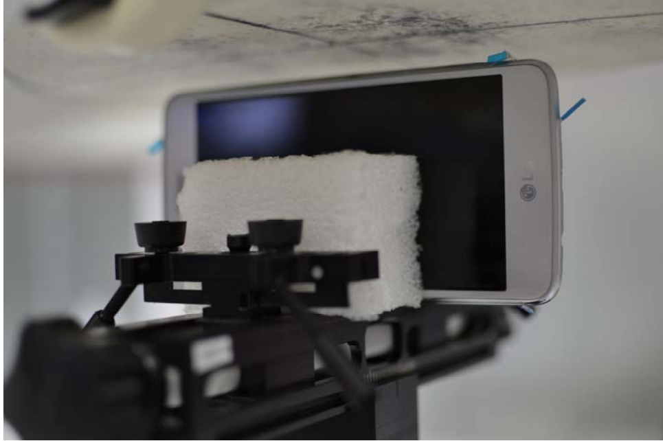
SAR Test Setup Photo 9: Right Edge at 10 mm
