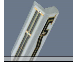
Figure 4-1 E-field Free-space Probe
