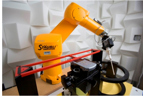
Figure 4-3 SPEAG Robotic System
