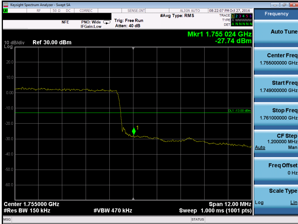
Plot 7-111. Upper Band Edge Plot (Band 4 – 15.0MHz QPSK – RB Size 75)
