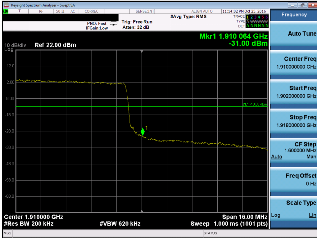
Plot 7-139. Upper Band Edge Plot (Band 2 – 20.0MHz QPSK – RB Size 100)
