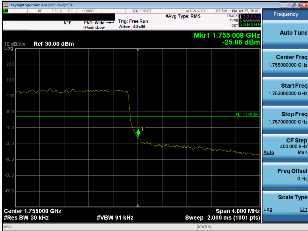
Plot 7-99. Upper Band Edge Plot (Band 4 – 3.0MHz QPSK – RB Size 15)
