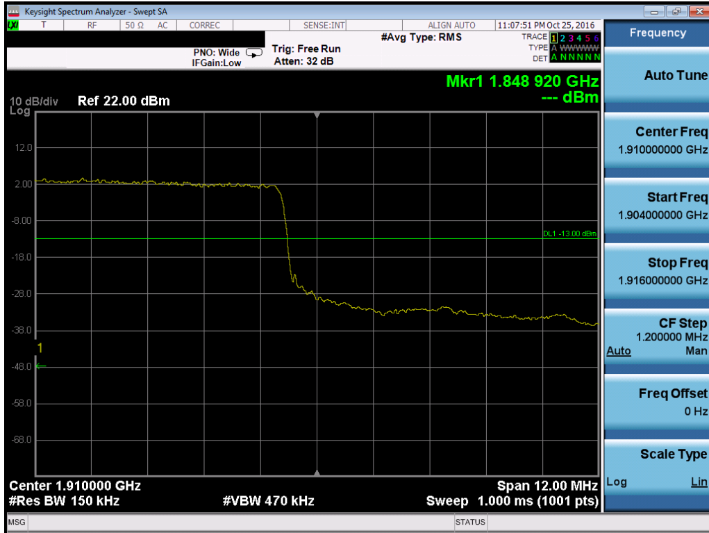
Plot 7-135. Upper Band Edge Plot (Band 2 – 15.0MHz QPSK – RB Size 75)
