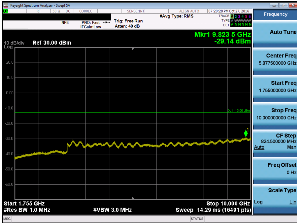
Plot 7-60. Conducted Spurious Plot (Band 4 – 10.0MHz QPSK – RB Size 1, RB Offset 0 – Low Channel)
