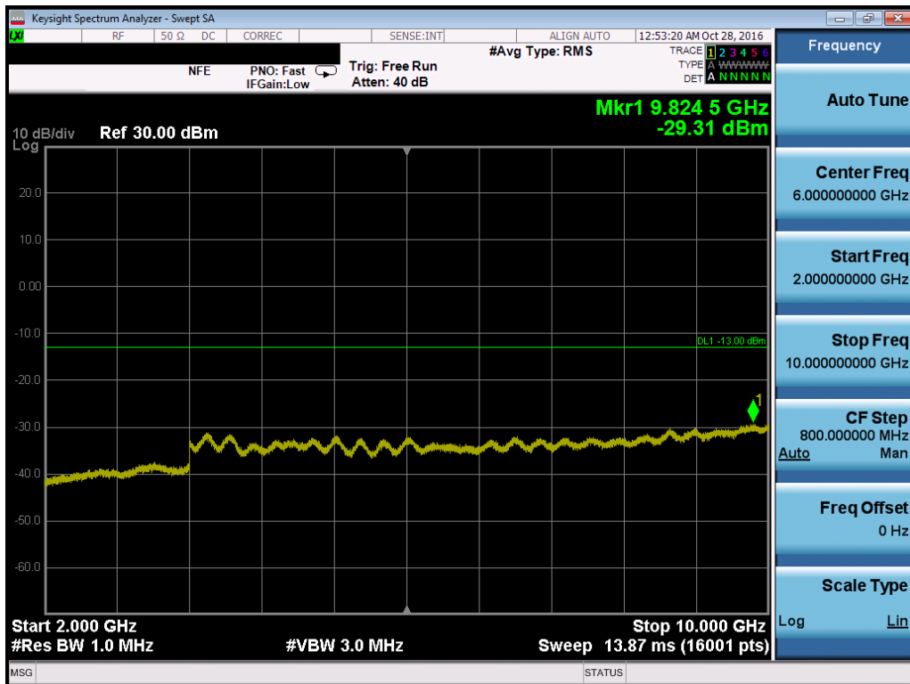
Plot 7-58. Conducted Spurious Plot (Band 5 – 1.4MHz QPSK – RB Size 1, RB Offset 0 – High Channel)
