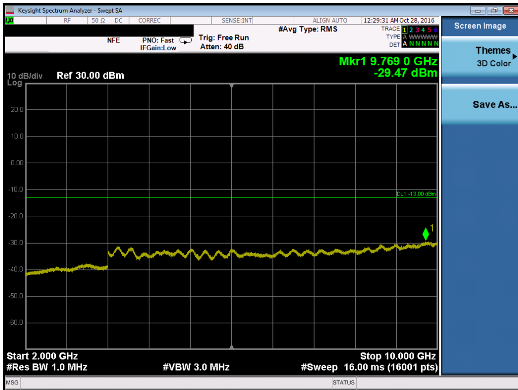
Plot 7-52. Conducted Spurious Plot (Band 5 – 1.4MHz QPSK – RB Size 1, RB Offset 0 – Low Channel)
