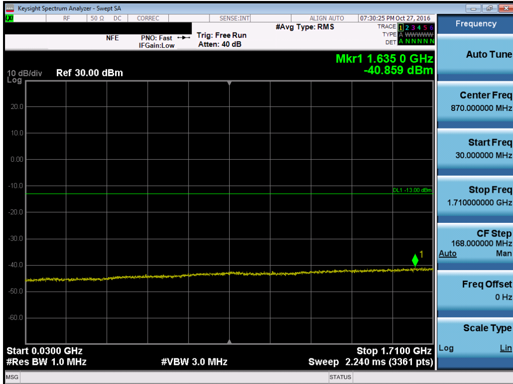
Plot 7-65. Conducted Spurious Plot (Band 4 – 10.0MHz QPSK – RB Size 1, RB Offset 0 – High Channel)
