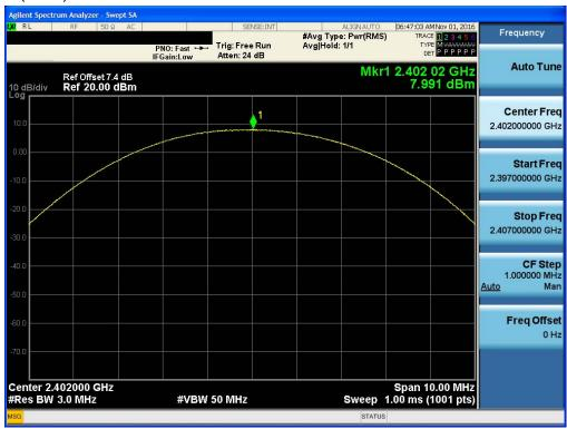
Test Plots ( $\pi/4DQPSK$ ) Peak Power (CH.39)
