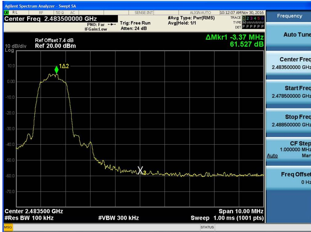
Test Plots with hopping (GFSK)
