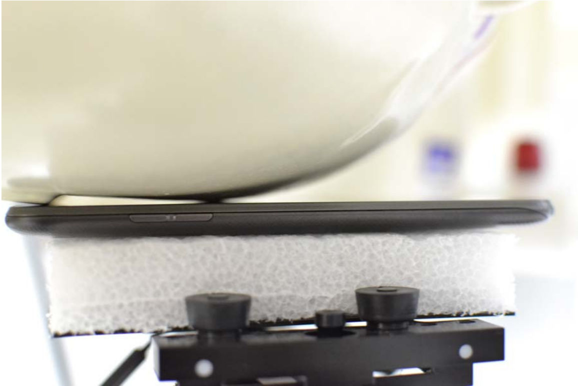
SAR Test Setup Photo 1: Right Cheek
