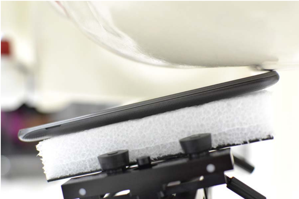
SAR Test Setup Photo 4: Left Tilt
