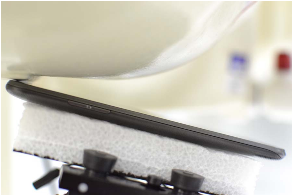
SAR Test Setup Photo 2: Right Tilt
