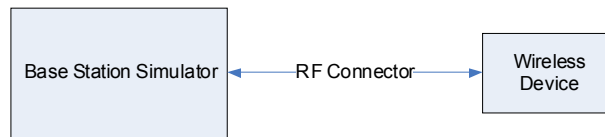
Figure 9-2 Power Measurement Setup
